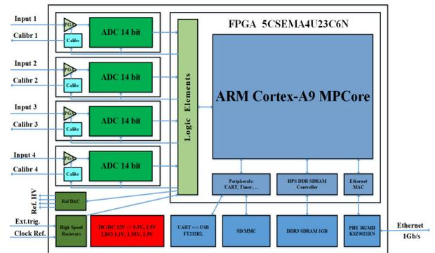
Figure 5: Measuring module for the CBLM (top), scheme of the CBLMs in successive segments of the magnetic structure (bottom).
