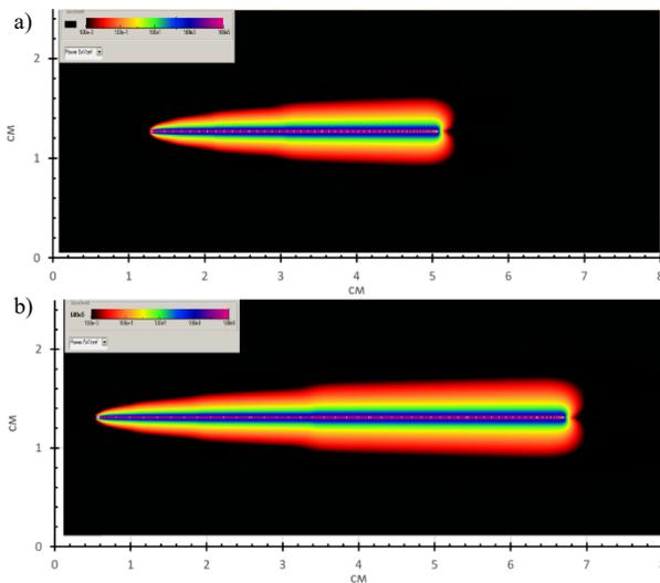
Figure 6: Synchrotron radiation of a DL1 dipole magnet, a) ESRF-EBS; b) USSR.
