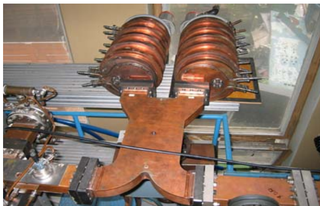
Figure 1: SLED energy compression system design from IREN (JINR, LNP).
