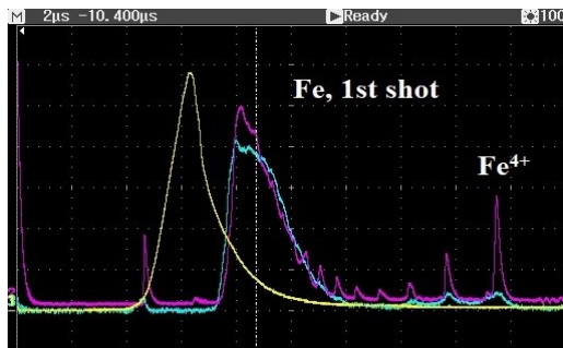
Figure 2: TOF spectrum of the ions at the output of the laser ion source, white vertical line is TOF marker for Fe^{16+} , lilac - SEM detector signals, blue - collected signal at the SEM input, yellow - collected signal at the analyzer input.
