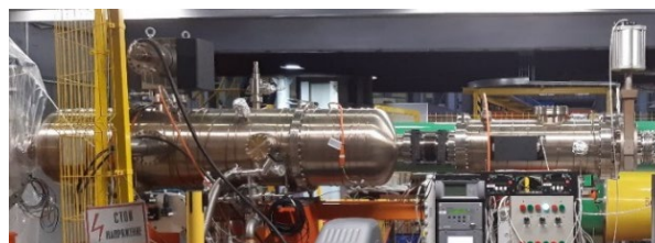
Figure 5: The electrostatic septum (left vacuum box) and the module of inflector plates IP2 (right vacuum box).
