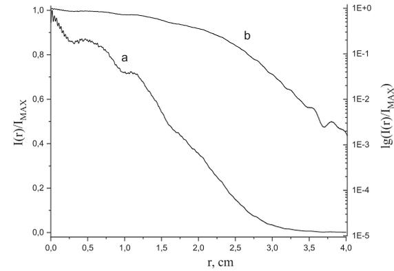
Figure 5: The calculated laser beam energy density distributions on the small mirror of the amplifier telescope. The spatial filter base detuning is -100 mm. a — in a linear scale; b — in a logarithmic scale.
