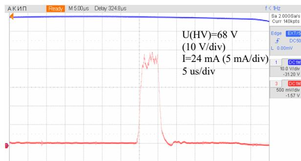
Figure 10: Signal Faraday Cup at LEBT (red), signal from divider of the HV pulsed transformer (blue).
