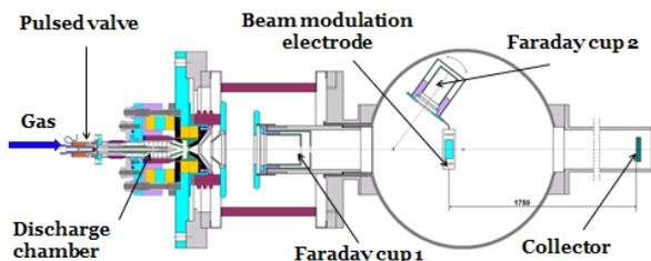
Figure 5: Test bench layout for the TOF measurements.
