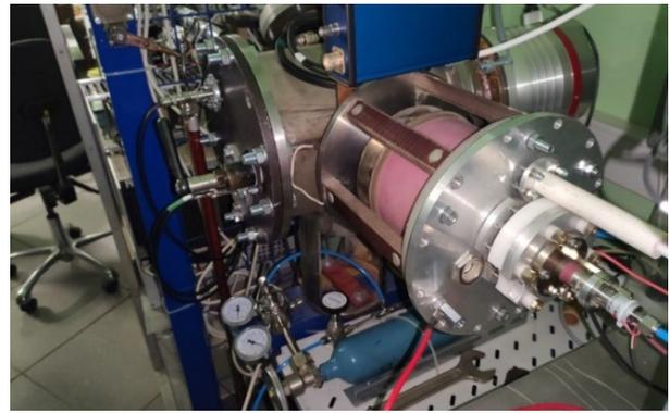
Figure 6: Helium ion source at the test bench.
