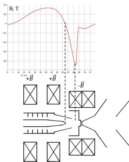
Figure 2: Equivalent diagram and graph of the magnetic field distribution along the axis.
