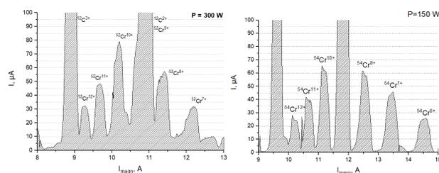
Figure 11: The <sup>52</sup>Cr (left) and <sup>54</sup>Cr (right) ion spectra, optimized for Cr<sup>10+</sup>.
