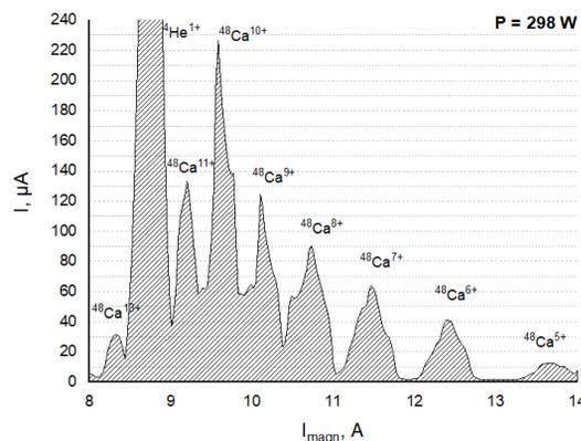
Figure 7: The  $^{48}\text{Ca}$  ion spectrum, optimized for  $\text{Ca}^{10+}$ .
