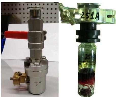
Figure 9: Containers with: left - (CH<sub>3</sub>)<sub>5</sub>C<sub>5</sub>Ti(CH<sub>3</sub>)<sub>3</sub> and right – C<sub>10</sub>H<sub>10</sub>Cr.
