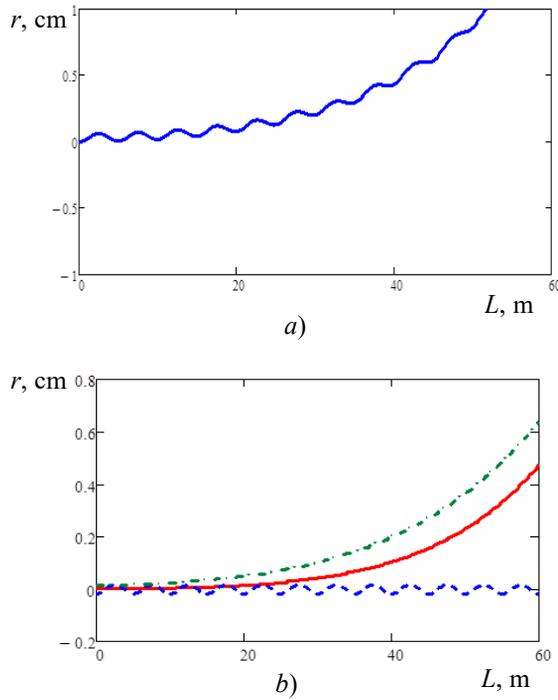
Figure 2: Results of modelling the beam dynamics for the cosine dependence of the waveguide bending: *a*) the beam trajectory, *b*) the effect of individual terms (red solid line is  $r_{free}$ , blue dashed line – the first term of  $r_{cos}$ , green dash-dotted line – the second term of  $r_{cos}$ ).
