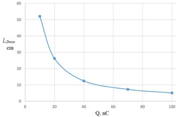
Figure 4: Dependence of  $L_{Dmax}$  on bunch charge.
