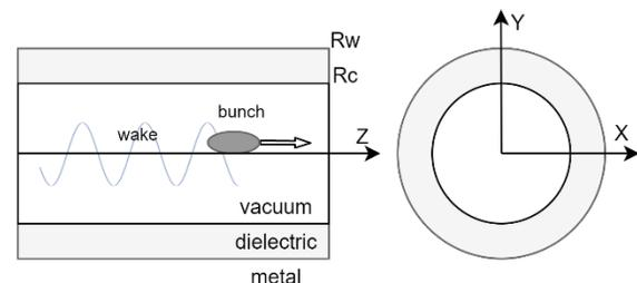
Figure 2: Dechirper based on cylindrical dielectric waveguide.
