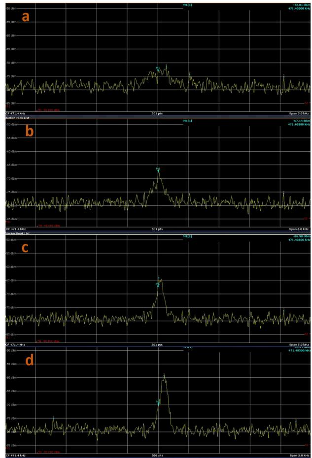
Figure 7: The signal from the Schottky spectrometer. a) is the signal of injection of an ion  $^{56}\text{Fe}^{14+}$  beam into the Booster ring, b), c), d) are the cooling of the ion beam by an electron beam.
