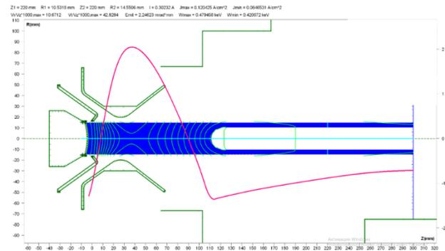
Figure 5: Formation of the hollow beam Potential values:  $\varphi_{cath} = -1.3$  kV,  $U_{an}=4$  kV,  $U_{grid} = 0.5$  kV. Longitudinal magnetic field is equal to 0.1 T. The red curve gives the electron beam potential distribution at the axis relatively to ground.
