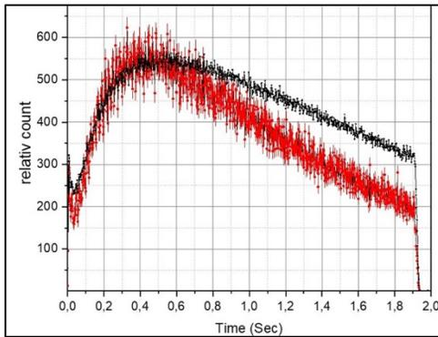
Figure 6:  $\langle RC(t) \rangle$  with the electron current off (black curve) and on (red curve). The electron energy is 1.78 keV, the electron beam current 150 mA. The latter is the optimum electron energy for electron cooling equal to  $(E_c)_{opt} = (m_e/m_{nucleon}) \times E_{ion}$ , where  $E_c$  is electron energy (not corrected to electron beam space charge potential!),  $E_{ion}$  is the ion energy per nucleon.
