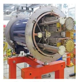
Figure 4: Collider dipole magnet.
