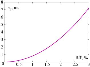
Figure 6: TLT vs energy acceptance (Q = 1 nC).
