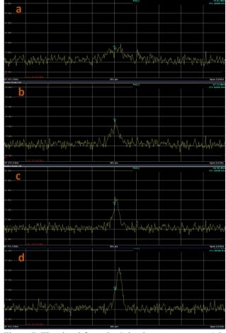
Figure 7: The signal from the Schottky spectrometer. a) is the signal of injection of an ion <sup>56</sup>Fe<sup>14+</sup> beam into the Booster ring, b), c), d) are the cooling of the ion beam by an electron beam.
