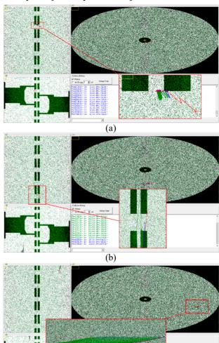
Figure 6: Example of the multipactor trajectories at a different voltage: (a) U=2.8 kV; (b) U=0.47 MV; (c) U=1.97 MV.
