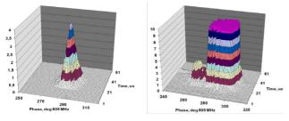
Figure 8: Observation of bunch longitudinal halo in the first SNS CCL: left – nominal SEM-gain, right – 160 times larger gain.
