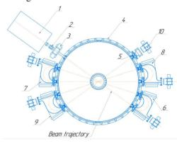
Figure 1: Accelerator scheme (1 – RF injector; 2 – focusing solenoid; 3 – quadrupole lens; 4 – accelerating cavity; 5 – corrector; 6 – 9 – bending magnets; 10 – Faraday cup).
