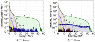
Figure 3: Secondary radiation energy spectra,  $E_{pr} = 60 \text{ MeV } (1 - p, 2 - \gamma, 3 - n, 4 - e^-, 5 - e^+, 6 - \alpha; 7 - \text{``other''}).$
