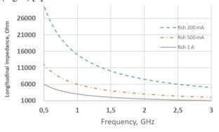
Figure 3: Threshold for longitudinal impedance necessary for unconditional beam stability for 200, 500 and 1000 mA beam current.
