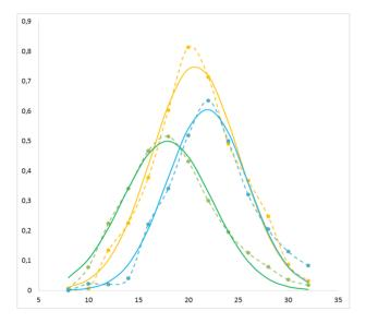
Figure 3: Profile of the proton beam passed through the peak of the beam. Solid line is approximation by the Gauss distribution, dash line are measured values. Yellow line is 1 mA, green one is 3 mA, blue one is 3 mA with a stronger focusing parameters.
