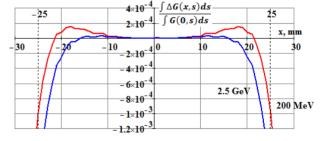
Figure 4: Integral homogeneity of the quadrupole field gradient.
