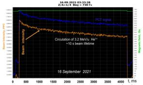
Figure 12: Beam current transformer signal at <sup>4</sup>He<sup>1+</sup> ion energy 3.2 MeV/u.
