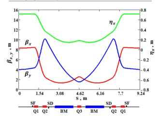
Figure 1: Twiss parameters for one booster cell.
