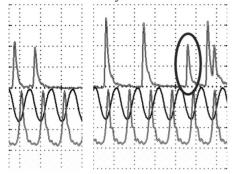
Figure 2: Oscillograms from the external detector: the upper line is a signal from external detector (2 divisions single proton events, 3 divisions – double protons event); the middle line is an accelerator RF; the bottom line is a beam current inside the synchrotron.
