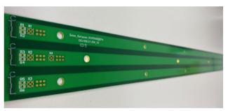
Figure 2: Block of the PCB harmonic coils.
