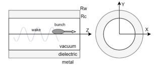
Figure 2: Dechirper based on cylindrical dielectric waveguide.
