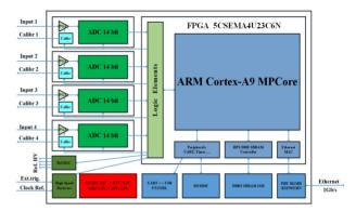
Figure 6: Measuring module for the SBLM.
