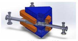
Figure 7: Dipole magnet 0.2 T.
