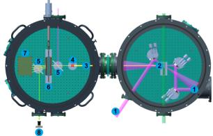
Figure 1: Experimental vacuum chamber. (1) Laser beams, (2) supersonic gas jet, (3) electronic beam, (4) RF beam charge detector, (5) screens, (6) magnet spectrometer, (7) faraday cap, (8) CCD.
