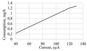
Figure 8: Calcium consumption as a function of Ca<sup>10+</sup> intensity.
