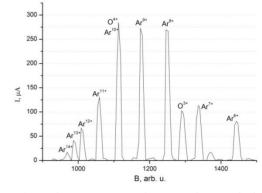
Figure 6: Ar ion spectrum. The operating mode is optimized to produce <sup>40</sup>Ar<sup>12+</sup>. Microwave power 309 W.
