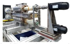
Figure 3: Warm magnetic measurement stand.
