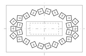
Figure 1: Quad formed with 26 identical 11 mm ×11 mm PM bricks each magnetized to 1.1402T. Arrows indicate PM orientations, dashed lines bound 64mm × 25mm working region, solid lines are for 80mm × 32mm aperture and 170mm × 106mm overall sizes.
