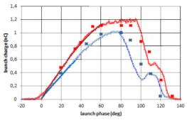
Figure 7: RF lunch phase influence.  $E_{cathode,max}$ =62 MV/m (red curve) and  $E_{cathode,max}$ =47.6 MV/m (blue curve). Crosses mark the SUMA calculation results.
