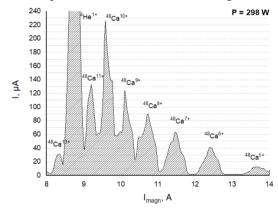
Figure 7: The <sup>48</sup>Ca ion spectrum, optimized for Ca<sup>10+</sup>.
