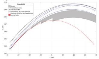
Figure 6: Graph of losses of ion beam <sup>209</sup>Bi<sup>38+</sup> in an electrostatic deflector with a constant gap.
