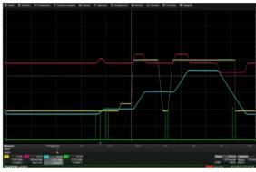
Figure 9: RF voltage applied to the falling magnetic field.
