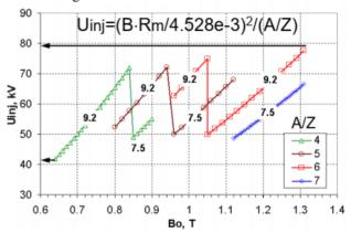
Figure 1: Dependence of the magnetic field on the injection voltage for the inflector A and B.
