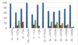
Figure 3: Calculated contributions of hadrons to the reaction rates in %. Neutrons contribution shows by blue colours, protons – red, pions – green.
