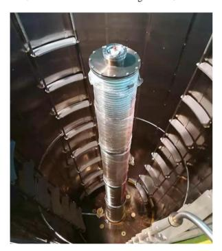
Figure 2: The ELV-15 accelerating tube.
