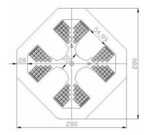
Figure 3: The quadrupole cross section.
