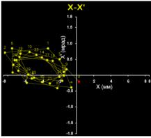
Figure 6: Phase trajectories of horizontal coherent oscillations of the injected Fe<sup>14+</sup> beam at the exit of the electrostatic septum. Red point is the calculated initial position of the injected beam. Phase coordinates are given in mm and mrad.
