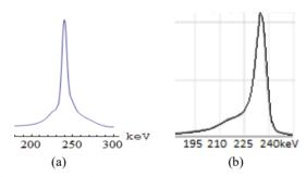
Figure 8: (a) - The spectrum from the absorbing filters method.; (b)- The spectrum on a magnetic spectrometer.
