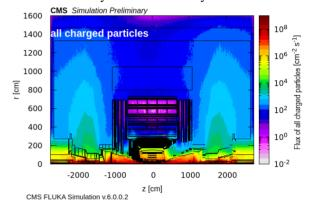
Figure 1: MC estimation of the flux of all charged particles in the CMS detectors and cavern at nominal HL-LHC luminosity  $5 \times 10^{34}$  cm<sup>-2</sup>s<sup>-1</sup>.
