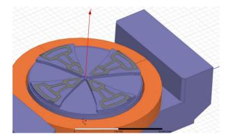
Figure 3: 3D calculation model of 1/2 electromagnet with azimuth coil housings.
