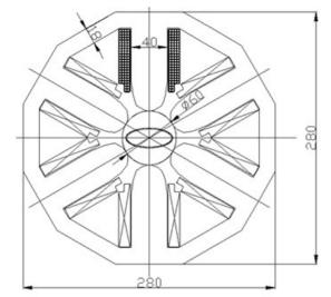
Figure 5: The sextupole cross section.
