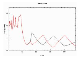
Figure 6: Beam transverse size evolution in the linac.
