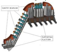
Figure 4: Layout of the gantry beamline and support platforms for magnetic elements.
