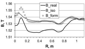
Figure 2: Operational formation of the magnetic field for 209Bi38+ acceleration mode.
