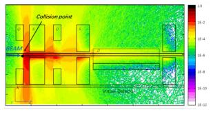
Figure 3: Typical distribution of the secondary charged particles for the beam loss in the SKIF lattice.
