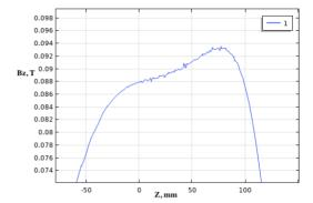
Figure 6: Axial magnetic field profile of the microwave source operating mode with the adjustable position of the ring magnets.
