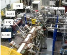
Figure 1: New fore-injector for LU-20.
