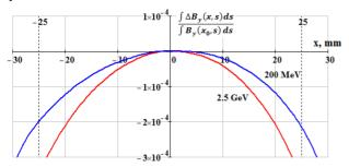
Figure 2: Integral homogeneity of the dipole field.
