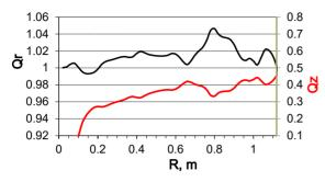
Figure 3: Radial and vertical betatron oscillation frequencies for 209Bi38+ acceleration mode.
