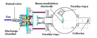
Figure 5: Test bench layout for the TOF measurements.
