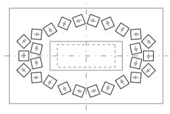
Figure 9: Cross section of PMQ consisting of 26 permanent magnets.
