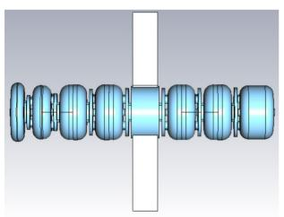
Figure 5: Side view of the S-band accelerating structure with the power coupler.
