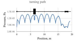
Figure 10: Pressure distribution in the HEBT channels.
