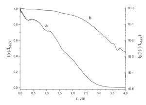
Figure 5: The calculated laser beam energy density distributions on the small mirror of the amplifier telescope. The spatial filter base detuning is -100 mm.
