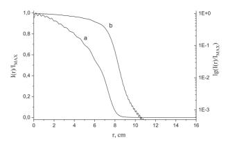
Figure 4: The calculated laser beam energy density distributions at the amplifier output. The spatial filter base detuning is +80 mm.
