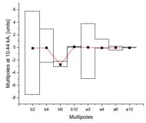
Figure 12: Multipoles for quadrupole magnets of the NICA project.
