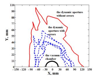
Figure 3: Dynamic aperture for the booster lattice.
