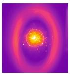
Figure 7: Image obtained from the infrared camera during the target irradiation by a proton beam with a current of 1.4 mA. The dashed circle denotes the diameter of 30
