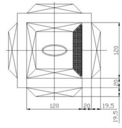
Figure 7: The corrector cross section.
