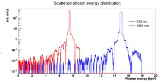
Figure 4: Geant4 simulation of ICS. Head-on collision of the 20 MeV electron beam with a laser beam with wavelengths of 532 (blue) and 1064 (red) nm, pulse time is 9 ns,  $a_0 = 0.03$ , observation angle  $\theta$  is 3 mrad relative to the initial trajectory of electrons.
