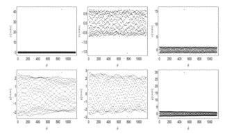
Figure 2: Examples of spike anomalies in TbT signals. Spikes appear in both planes.
