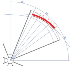
Figure 7: Layout of the magnetic channel in the cyclotron extraction system.
