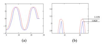
Figure 7: Dimensionless amplitude of the accelerating field  $\hat{e} = eE / 2\pi W_0$  in the center of the cell before the first bunch pass (red curve) (a) and taking into account the introduced disturbance (b).
