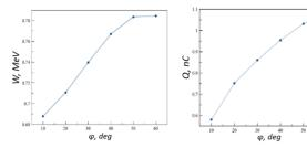
Figure 2: Left – dependence of the electron average energy on the injection phase, right – bunch charge dependence on the injection phase.
