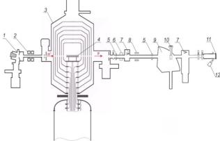
Figure 1: A diagram of an accelerator based source of epithermal neutrons. 1 - H<sup>-</sup> source, 2 - magnetic lense, 3 - vacuum-insulated tandem accelerator, 4 - gas stripping target, 5 - cooled diaphragm, 6 -NPCT contactless beam sensor (Bergoz, France), 7 - movable Faraday cup 8 - corrector, 9 - bending magnet, 10 - cooled beam receiver with a diaphragm, 11 - lithium target, 12 - Hikvision video camera.
