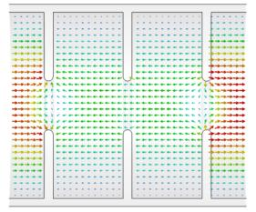
Figure 3: Distribution of accelerating field on mode  $2\pi/3$  in the model.
