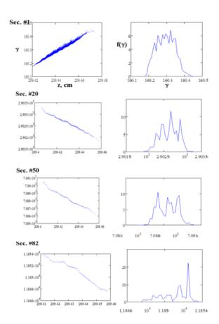
Figure 6: Beam dynamics simulation results in regular part of accelerator-injector for bunch with 250 pC charge, generated by RF photogun. Phase portraits on the phase plane  $(\gamma, z)$  and the energy spectrum.
