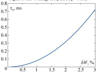
Figure 7: TLT vs energy acceptance (Q = 100 pC).
