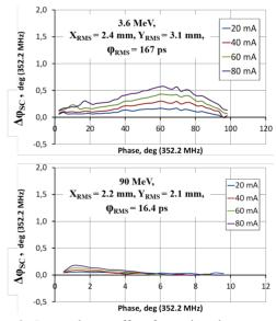
Figure 2: Space charge effect for various beam currents.
