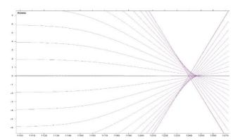
Figure 7: Simulation of the beam trajectories at final focusing lens.
