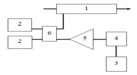
Figure 2: Block diagram of LINAC with an energy compression system SLED (1 - accelerating section, 2 - storage resonators, 3 - master oscillator, 4 - high-speed phase shifter, 5 - power amplifier, 6 - high frequency bridge).
