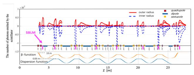
Figure 4: The simulated distribution of optical photons in the scintillator over the SKIF storage ring superperiod. The sign of the vertical axis only has meaning of direction.
