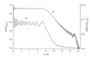
Figure 6: The calculated laser beam energy density distributions at the amplifier output. The spatial filter base detuning is -100 mm.
