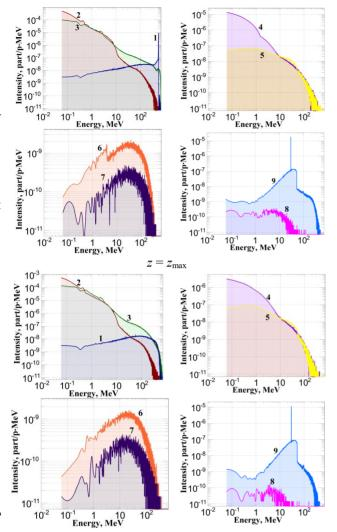
Figure 4: Secondary radiation energy spectra,  $E_{pr} = 700 \text{ MeV } (1 - p, 2 - \gamma, 3 - n, 4 - e^-, 5 - e^+, 6 - \mu^+, 7 - \mu^-, 8 - \alpha, 9$  "other").
