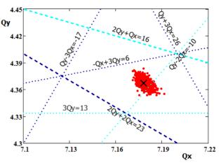
Figure 2: The betatron tunes diagram: the black cross – tunes for the lattice without errors, read points – tunes for the lattice with 1000 sets of random errors.
