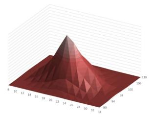
Figure 2: Result of the two-dimensional tomography for the proton current 1.2 mA. X and y axes are coordinates of the diaphragm, z axis is current distribution.
