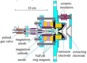
Figure 1: Helium ion source design.
