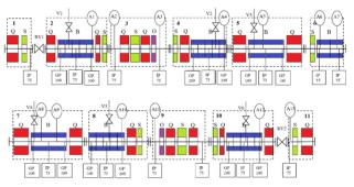
Figure 1: Standard cell: vacuum chambers 1-11, vacuum pumps IP and GP, absorbers A1-13.
