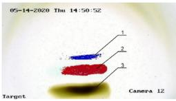
Figure 2: Images from a video camera looking at the surface of a lithium target at a bending magnet current of (a) 0 and (b) 14 A and (c) 14 A with partially inverted colors. 1, glow caused by neutrals (hydrogen atoms); 2, argon ions; 3, protons.
