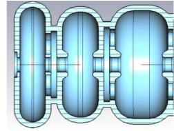
Figure 2: Sectional side view of the bunching part.
