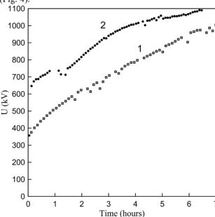
Figure 4: Graphs of the first increase in voltage at the accelerator after modernization: 1 - smooth ceramic, 2 - ribbed ceramic.
