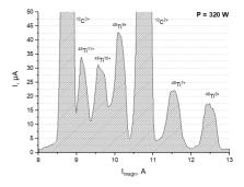
Figure 10: The <sup>48</sup>Ti ion spectrum, optimized for Ti<sup>10+</sup>.
