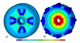
Figure 2: RF loss density (a) and temperature (b) distributions in CDS.
