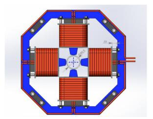
Figure 1: Front view of the pulse quadrupole.
