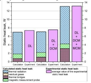
Figure 2: Comparison of the calculated and experimental value of static heat leak for different configurations of the Booster quadrupole magnets.
