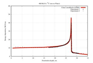
Figure 8: The total absorbed dose versus depth inside water phantom at 400 MeV/u of incident <sup>12</sup>C beam (R<sub>csda</sub>=27.135 g/cm<sup>2</sup>).
