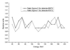
Figure 5: Ratio of measured values for beam σ at X and Y axes.
