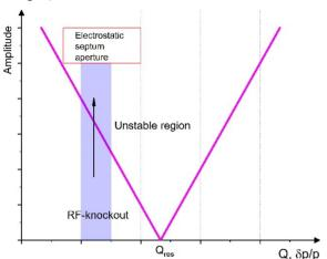
Figure 3: Steinbach diagram show RF-knockout driving mechanism.
