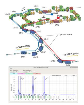
Figure 4: Beam loss monitor layout.
