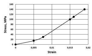
Figure 3: Strain-stress dependence of the superconducting coil of the quadrupole FFS.
