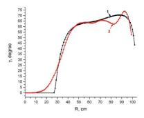
Figure 4: The spirality angle  $-\gamma$  (deg.) in dependence on the radius of the cyclotron: 1 - the data of the sector geometry spirality, 2 - the spirality of the fourth focusing harmonic of the magnetic field, obtained in 3D calculations and measurements of the magnetic field.
