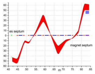
Figure 5: Spill position between electrostatic and magnet septums.
