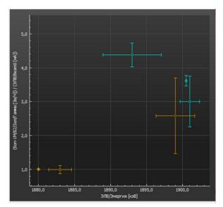
Figure 2: Gamma/Beam current VS Energy with standard deviation
