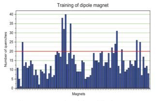
Figure 5: Cryogenic training of dipole magnets.
