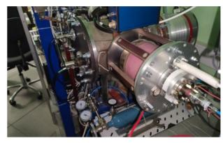
Figure 6: Helium ion source at the test bench.
