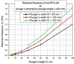
Figure 7: The resonant frequency dependence on plunger's dimensions.
