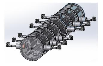
Figure 3: RFQ cavity design.
