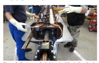
Figure 3: Equipment for baking the SC winding for the NICA collider dipole magnet.
