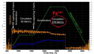
Figure 11: Beam current transformer signal at <sup>56</sup>Fe<sup>14+</sup> ion acceleration.
