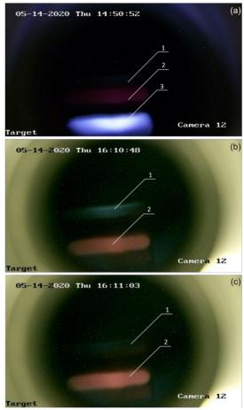
Figure 4: The glow recorded by a Hikvision video camera when a lithium target is irradiated with the components of a charged particle beam, at a bending magnet current of 14 A (a), 68 A (b) and 68 A and double gas injection into a stripping target (c). I, glow caused by neutrals (hydrogen atoms); 2, argon ions; 3, protons.
