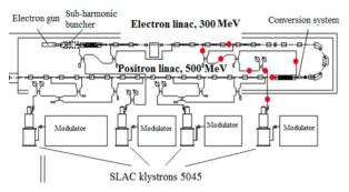
Figure 5: Measurement point layout of linac RF system.
