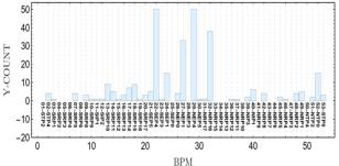
Figure 5: Flagged BPMs for 50 successive measurements. BPMs with high counts correspond to systematic anomalies.
