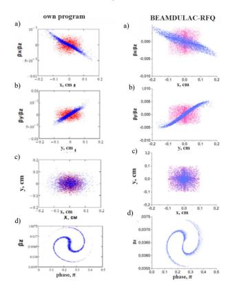
Figure 4: Results of O<sup>5+</sup>dynamics simulation: on the left in your own program; on the right - BEAMDULAC-RFQ (red dots - particles at the beginning of acceleration, blue dots - particles at the end of acceleration. a, b - transverse phase portraits; c - bunch cross-section; d - longitudinal phase portrait.
