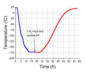
Figure 3: The time dependence of temperature in the center of the cryomodule during the first LN<sub>2</sub> tests.
