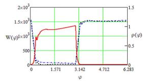
Figure 11: Longitudinal distribution (solid red line); RF potential - black dash-dotted line; total Self-Consistent Potential - blue dash-dotted line.
