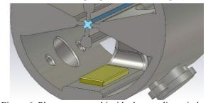
Figure 6: Plunger mounted inside the coupling window.
