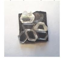
Figure 1: Synthetic crystal diamond plates.
