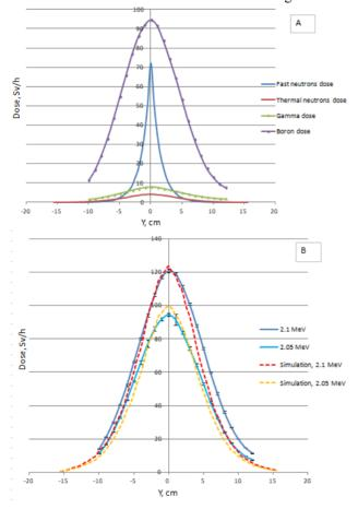
Figure 3: Distribution of doses along the Y-axis: the distribution of all doses (a), the comparison of experimental and calculated data of boron dose (b).
