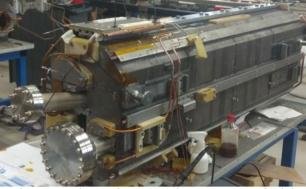
Figure 17: The Nuclotron Lambertson magnet for injection section.
