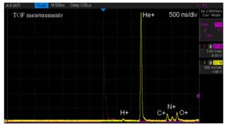
Figure 7: TOF spectrum obtained at the test bench for the helium ion source.
