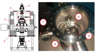
Figure 5: "Gun-collector" test bench (left) and diagnostic node of the test bench (right). 1 – electron gun, 2 – electron collector, 3 – solenoid, 4 – vacuum chamber, 5 – diagnostic node, 6 – wire support of the monitor, 7 – electric feedtroughs for the monitor, 8 – tube for vacuum window, 9 – BPM.
