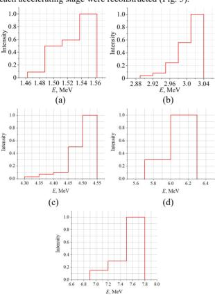
Figure 5: Reconstructed electron energy spectrum after one (a), two (b), three (c), four (d) and five (e) passes of accelerating cavity
