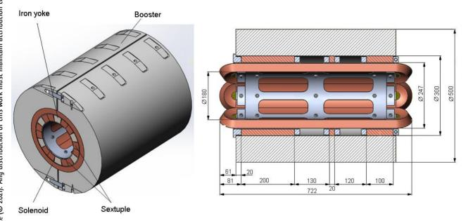
Figure 6: Conceptual design of magnetic system.
