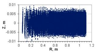
Figure 9: Vertical dimension of 209Bi38+ beam during acceleration from cyclotron center to extraction radius
