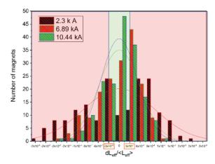
Figure 6: Arc dipole magnet distribution related to their effective lengths.
