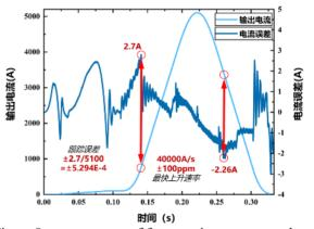
Figure 8: current curve of fast ramping power supply.
