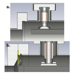
Figure 4: The design of the feedback kicker a) initial model and b) modified.
