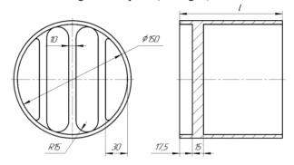
Figure 2: Vacuum port diagram.
