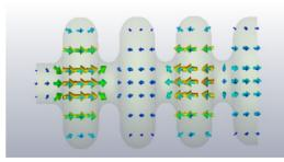
Figure 2: 3.5-cell RF-gun view and electrical field distribution.
