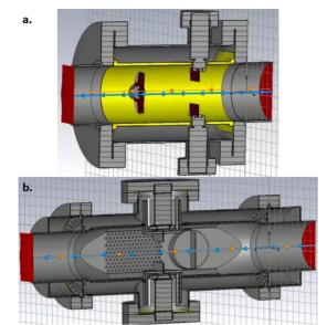
Figure 2: The design of the scraper a) initial model and b) modified.
