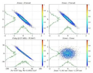
Figure 14: Output 238U<sup>61+</sup> beam particle distribution.
