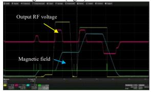
Figure 7: RF station parameters during adiabatic beam capture
