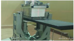
Figure 4: The 6-axis table in the medical module.
