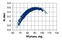
Figure 6: The distribution of ions energy in 209Bi38+beam at first orbit after injection.
