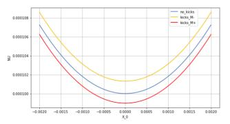
Figure 2: Spin-tune for different transversely offset particles for ideal lattice and with magnet tilts around the longitudinal axis  $\varphi \sim N(\pm 10^{-3}, 10^{-4})$ .
