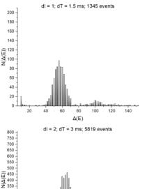
Figure 5: Samples of experimental measurements: the top diagram corresponds the first experimental series, the bottom one – the second series; these diagrams show the total number of detected events (including single protons, from
