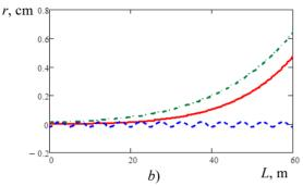
Figure 2: Results of modelling the beam dynamics for the cosine dependence of the waveguide bending: a) the beam trajectory, b) the effect of individual terms (red solid line is  $r_{free}$ , blue dashed line – the first term of  $r_{cos}$ , green dash-dotted line – the second term of  $r_{cos}$ ).
