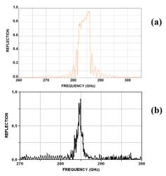
Figure 3: Results of (a) 3D simulations and (b) "cold" tests of advanced Bragg structure having oversize factor  $\emptyset/\lambda \sim 20$  and operating at 0.3 THz band (feedback loop TE<sub>1,1</sub>  $\leftrightarrow$  TE<sub>1,20 - cutoff</sub>  $\leftrightarrow$  TE<sub>1,1</sub>, length  $l_{\rm ad} = 10$  cm, corrugation period  $d_{\rm ad} = 1.05$  mm and depth  $r_{\rm ad} = 0.3$  mm).
