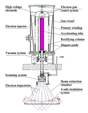
Figure 1: The ELV type accelerator view.
