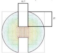
Figure 5: Distribution of TE11 mode electric field in a corrugated cylindrical waveguide.
