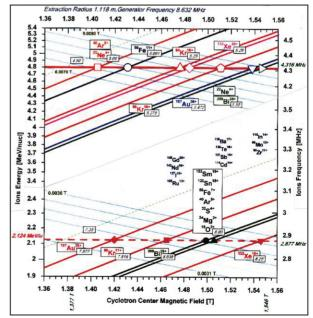
Figure 2: Working diagram of DC140 cyclotron.
