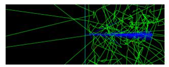
Figure 1: Trajectories visualization in Geant4. Neutral particle tracks shown in green, positively charged particle tracks shown in blue, negatively charged particle tracks shown in red, cyan line marks water phantom boundary.
