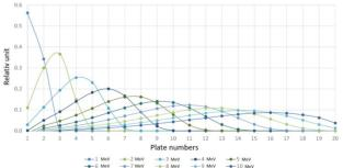
Figure 2: Spectral response of 20 plates assembly.
