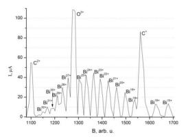
Figure 7: Bi ion spectrum. The operating mode is optimized to produce <sup>209</sup>Bi<sup>27+</sup>. Microwave power 220 W.
