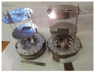
Figure 3: Photo of the two MCP-based detectors installed at the Booster for X and Y profile measurement.
