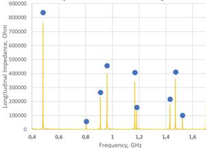
Figure 2: Frequency dependence of the longitudinal shunt impedance for monopole modes for an accelerating cavity at 357 MHz. Graph – result of wakefield simulations, dots - results of eigenmode simulations.
