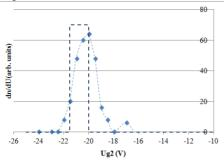
Figure 3: Measured spectrum of electrons with the gun accelerating voltage of 20 eV.  $U_{\rm g3} = -10$  V. The dashed line is the expected electron spectrum; the points are results of the measurements. Temperature of the TGA was  $100^{\circ}$ C.
