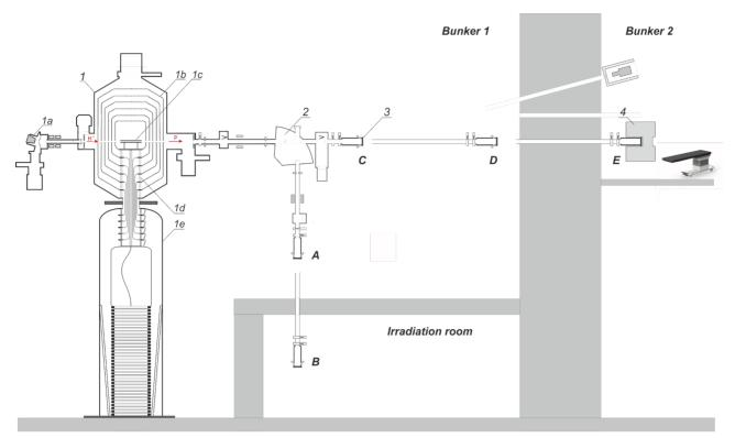
Figure 1: Layout of the experimental facility: 1 – vacuum-insulated tandem accelerator (1a – negative ion source, 1b – intermediate- and high-voltage electrodes, 1c – gas stripper, 1d – feedthrough insulator, 1e – high-voltage power supply), 2 – bending magnet, 3 – lithium target, 4 – beam-shaping assembly. A, B, C, D, E – lithium target placement positions.
