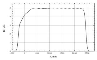
Figure 3: Designed magnetic field profile of a new positron solenoid.
