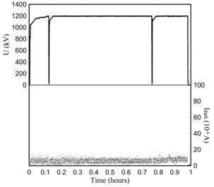
Figure 5: Graphs of the voltage U and dark current I dark at the accelerator versus time.
