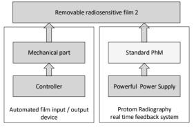
Figure 3: Low Intensity Beam Extraction Control System principle design.
