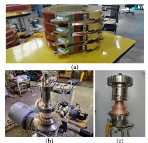
Figure 11: the coils, the gun and the collector for 450 keV cooler.
