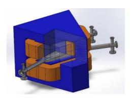
Figure 8: Dipole magnet 1.19 T.
