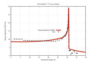
Figure 9: The total absorbed dose versus depth inside water phantom at 430.10 MeV/u of incident <sup>12</sup>C beam (R<sub>csda</sub>=30.463 g/cm<sup>2</sup>).
