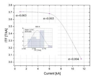
Figure 6: Current dependence of Integral transfer functions of the quadrupoles. The inset graph gives der distribution for 22 series magnets at 900 A.
