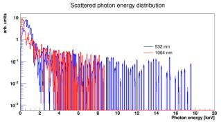
Figure 5: Geant4 simulation of ICS. Collision of the 20 MeV electron beam with a laser beam with wavelengths of 532 (blue) and 1064 (red) nm, pulse time is 9 ns,  $a_0 = 0.03$ , collision angle  $\alpha = 7^{\circ}$ , observation angle  $\theta$  is 3 mrad relative to the initial trajectory of electrons.
