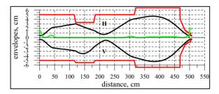
Figure 8: Horizontal (H) and vertical (V) <sup>197</sup>Au<sup>26+</sup> beam envelopes, aperture (red line) and longitudinal magnetic field (green line).
