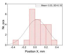
Figure 5: The defocusing quadrupoles normal distribution of the X positions of the magnetic center.
