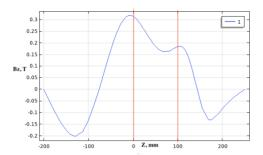
Figure 4: Magnetic flux density distributions of the system with the solenoids. The red lines depict the plasma chamber boundaries.
