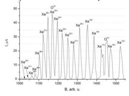
Figure 4: Xe ion spectrum. The operating mode is optimized to produce <sup>132</sup>Xe<sup>27+</sup>. Microwave power 290 W.
