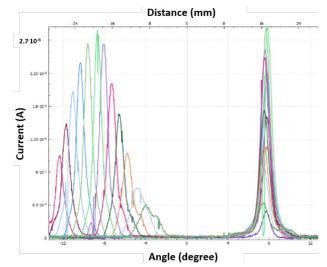
Figure 2: Beam measurements along one coordinate made by wire scanner.
