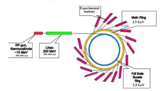
Figure 1: Planned scheme of the accelerator complex.
