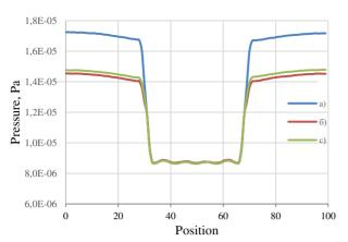
Figure 8: Pressure distribution along the axis of the resonator and pipelines.
