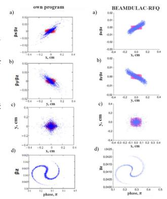
Figure 3: Results of proton dynamics simulation: on the left - in your own program; on the right - BEAMDULAC-RFQ (red dots - particles at the beginning of acceleration, blue dots - particles at the end of acceleration). a, b - transverse phase portraits; c - bunch cross-section; d - longitudinal phase portrait.
