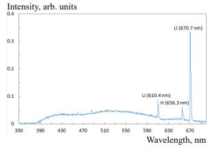
Figure 2: The luminescence spectrum of the lithium target.
