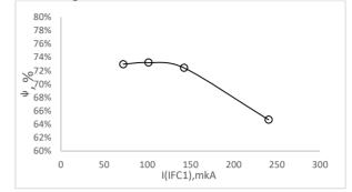
Figure 3: The efficiency of capture into acceleration.
