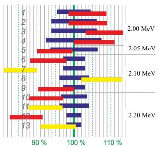
Figure 4: The result of the study comparing the measured neutron yield with the calculated one: from top to bottom-targets in order, blue rectangles - intervals of the calculated number of neutrons, red and yellow – intervals of the measured number of neutrons (red – natural lithium, yellow – enriched with lithium-7 isotope). On the right are the characteristic values of the proton energy.
