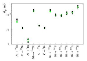
Figure 4: The neutron reactions cross sections weighted by the calculated fluence spectra at three points. Green points correspond to 10 GeV proton beam, black - 50 GeV.  $(\bullet, \bullet - p. 1; \circ, \circ - p. 2; \blacktriangle, \blacktriangle - p. 3)$ .
