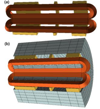
Figure 1: Conventional (sextupole-in-solenoid) magnetic system. Model without (a) and with (b) iron.
