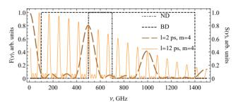
Figure 4: Form-factors of electron trains for two bunch spacing (both TR and DR cases are coincides) and detector sensitivity ranges for both ND and BD cases.
