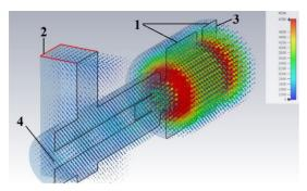
Figure 2: RF photogun layout (1-accelerating cavities; 2-RF power input; 3-cavity wall with a photocathode; 4-cavity for laser input and beam output).
