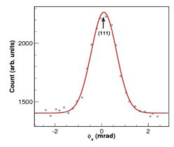
Figure 6: C<sub>1</sub> counting rate depending on the horizontal angle of crystal rotation.
