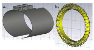
Figure 7: a) Shielding "clamp" and b) "springs".
