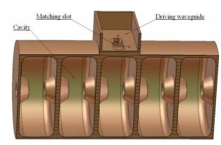
Figure 1: Schematic drawing of the cavity - slot - WG system to be matched.
