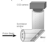
Figure 2: Scheme of scintillation detector.
