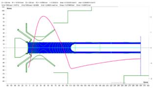
Figure 5: Formation of the hollow beam Potential values:  $\varphi_{cath} = -1.3 \text{ kV}$ ,  $U_{an} = 4 \text{ kV}$ ,  $U_{grid} = 0.5 \text{ kV}$ . Longitudinal magnetic field is equal to 0.1 T. The red curve gives the electron beam potential distribution at the axis relatively to ground.
