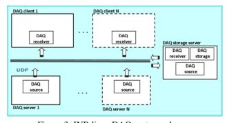
Figure 3: INR linac DAQ system scheme.
