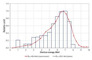
Figure 6: Electron energy spectrum, obtained with the aid of magnet spectrometer and by absorbing filter method.
