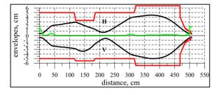
Figure 6: Horizontal (H) and vertical (V) <sup>209</sup>Bi<sup>38+</sup> beam envelopes, aperture (red line) and longitudinal magnetic field (green line).
