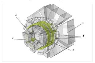
Figure 3: The model of the ECR mode magnetic system. (1) Injection ring magnet. (2)Middle ring magnets. (3) Extraction ring magnet. (4) Hexapole magnet. (5) Solenoids.
