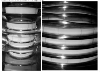
Figure 2: Smooth ceramic surface after training (left, right) with breakdown traces.
