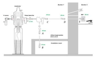
Figure 4: Estimated beam size at different positions of the lithium target.
