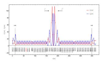
Figure 1: The VEPP-4M lattice functions.
