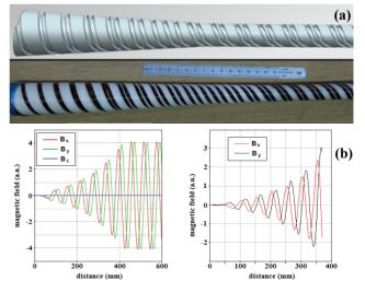
Figure 2: (a) Photograph of 3D model (top) and experimental prototype (bottom) of the "improved" undulator with a period  $d_{\rm u}=6$  cm, and (b) results of 3D simulations (left) and "cold" measurements (right) of longitudinal structure of magnetic field at the undulator entrance.
