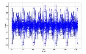
Figure 6: Horizontal orbit distortions,  $\sigma_{x/y}$  is 50  $\mu$ m.
