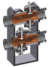
Figure 6: Horizontal and vertical collimator design for two-level collider rings.
