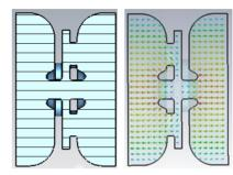
Figure 3: General view of regular section and electric field distribution.
