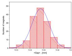
Figure 10: Interpolar gap for dipole magnets of the NICA project.
