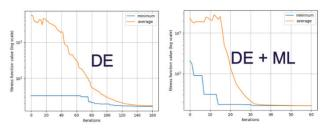
Figure 5: Comparison of the evolution of average (orange) and minimum (blue) fitness (KSRS emittance) without (left) and with (right) machine learning.
