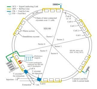
Figure 1: Scheme of the six sections of the synchrotron ring with Bypass Lines, the cryogenic and electrical supply systems.
