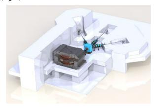
Figure 7: Layout of the cyclotron system main equipment (project).
