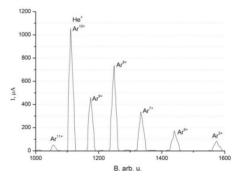
Figure 5: Ar ion spectrum. The operating mode is optimized to produce <sup>40</sup>Ar<sup>8+</sup>. Microwave power 274 W.
