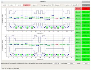
Figure 4: Displaying damping ring beam position. Green marker is the last measured beam coordinate, blue marker is the saved position, red is the inactive BPM's.
