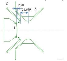
Figure 3: The Booster ECS gun scheme.
