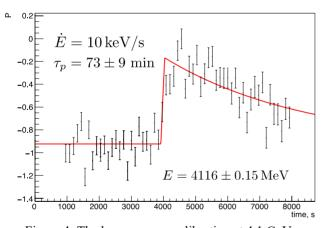
Figure 4: The beam energy calibration at 4.1 GeV.
