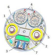
Figure 3: High-voltage section. 1 – electrostatic tube, 2 – magnetic coil, 3 – electronics unit, 4 – sections of cascade transformers, 5 – insulating supports, 6 – external ring, 7 – oil tubes.
