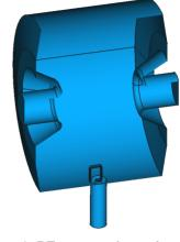
Figure 1: RF cavity with coupling loop.
