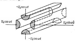
Figure 1: Quadrupole symmetric four-wire line.
