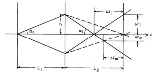
Figure 6: Schematic representation of particle trajectories when passing through a thin lens with spherical aberration.
