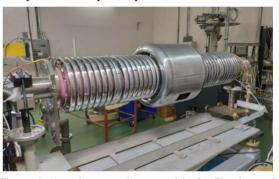
Figure 3: Accelerator tube assembly for Tandem v.2.
