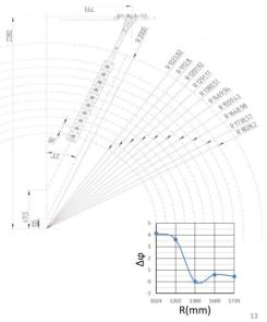
Figure 3: Placing of phase moving control system, and example of analisis for  $^{40}\text{Ar}^{+7}$  (F=8.51 Hhz; E=5.2 MeV/n).
