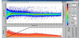
Figure 16: The size and beam intensity of extracted from Nuclotron Kr<sup>26+</sup> ion beam.
