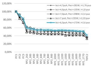
Figure 6: Comparison of normalized <sup>52</sup>Cr beam intensity in different points of cyclotron for different beam intensities.
