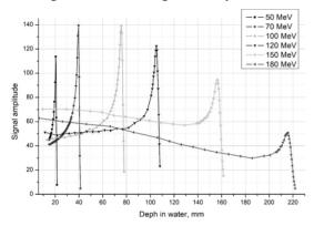
Figure 6: Bragg Peak curves measured by scintillation de-
