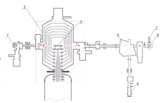
Figure 2: Experimental setup: I – negative hydrogen ion source, 2 - accelerator, 3 - argon stripping tube, 4 bending magnet, 5 – lithium target, 6 – vacuum chamber with cooled 45° mirror, 7 – telescope.
