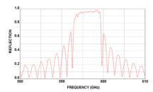
Figure 4: Results of 3D CST simulations of advanced Bragg structure with oversize factor  $D/\lambda \sim 40$  in the frequency band of 0.6 THz ( $l_{\rm ad} = 7.5$  cm,  $d_{\rm ad} = 0.5$  mm,  $r_{\rm ad} = 0.3$  mm, feedback loop TE<sub>1,1</sub>  $\leftrightarrow$  TE<sub>1,40-cutoff</sub>  $\leftrightarrow$  TE<sub>1,1</sub>).
