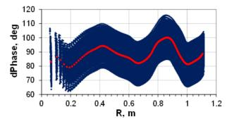
Figure 7: The phases of ions in 209Bi38+ beam during acceleration from cyclotron center to extraction radius.
