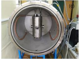
Figure 2: Niobium cavity inside of testing cryostat.
