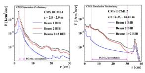
Figure 6: MC estimation of the radial distribution of the flux of all charged particles of BIB in CMS BCML1 (left) and BCML2 (right) detectors per one second of HL-LHC operation.
