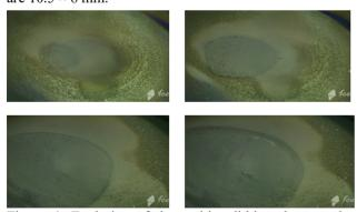
Figure 4: Evolution of the melting lithium layer under bombardment of the proton beam with 2 MeV energy. Upper left is 1.56 mA proton beam current, upper right is 1.81 mA, lower left is 2.59 mA and lower right is 3.05 mA.
