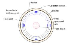
Figure 1: Schematic drawing of the TGA cross-section.
