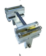
Figure 4: Crystalline undulator for a 6 GeV positron beam: a - its photograph and a schematic representation of its cross section (inset); b - appearance of the array of plates in one holder (crystal target in the assembly).
