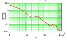
Figure 10: System impedance calculated by equivalent circuit impedance, Z<sub>out</sub>/n.
