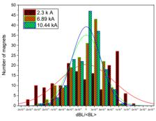
Figure 7: Relative spread of the integral of the magnetic field for dipole magnets of the NICA project.
