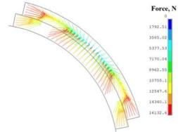
Figure 6: Distribution of pondemotive forces at the current of 5.73 kA in the coil quadrupole FFS.
