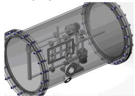
Figure 1: Discharge chamber for new laser ion (form Li to O) source.
