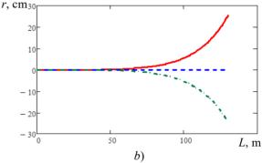
Figure 3: Beam dynamics simulation results with correction by introducing bias with sine ( $\chi = -0.085$ ).
