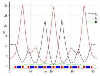
Figure 2: Lattice function of synchrotron quarter.
