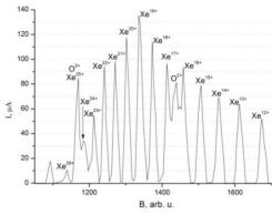
Figure 3: Xe ion spectrum. The operating mode is optimized to produce <sup>132</sup>Xe<sup>20+</sup>. Microwave power 308 W.
