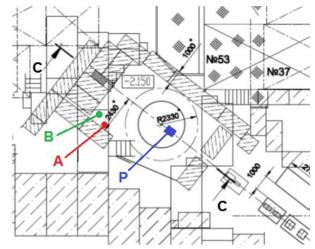
Figure 1: Schematic top view of the RBS facility. A and B – pair of the neutron monitors, C – ion beam, P – water phantom.
