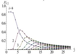
Figure 3: Distribution of absorbed charges overbeams of different energies for each plate i.
