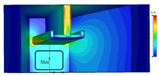
Figure 7: Distribution of tangential magnetic field at the inner surface in modified WG.
