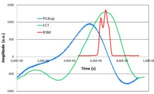
Figure 10: Bunch shapes of identical bunches of 3.5 Mev/u Ar9+ beam in GSI cw-Linac prototype measured with three different detectors.
