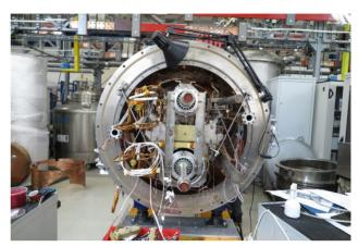
Figure 6: Assembly on a test cryostat for cryogenic testing.
