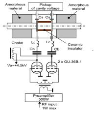
Figure 2: Block diagram of RF power amplifier.
