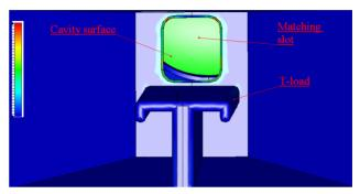
Figure 8: The resulting effect of T-load implementation – distribution of RF loss density in the total system near slot vicinity.
