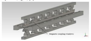
Figure 3: Electrodes with offset magnetic coupling windows
