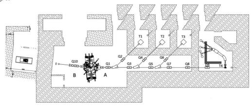
Figure 1: Blueprint of the project and beam transfer lines: (Right) A - beam line for radioisotope part, Q1-Q9 - lens doublets, T1-T4 - target stations. (Left) B - beam line for the ocular oncology complex, Q10 - triplet lenses.
