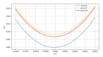
Figure 4: The dependence of a vertical component of the invariant axis  $N_y$  in the detector point for different transversely offset particles for ideal lattice and with magnet tilts around the longitudinal axis  $\varphi \sim N(\pm 10^{-3}, 10^{-4})$ .
