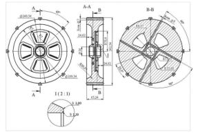
Figure 4: CDS structure design drawing at 991MHz operating frequency,  $\beta$ =0.4313.
