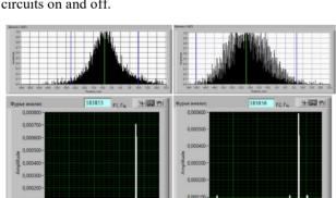
Figure 5: Horizontal profile (top) and Fourier analysis (bottom) with on (left) and off (right) feedback loops.
