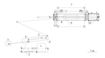
Figure 1: Experimental setup. 1 — master oscillator; 2 — absorbing cell; 3 — diffraction grating; 4 — short-focus mirror of the spatial filter; 5 — spatial filter diaphragm; 6 — long-focus mirror of the spatial filter; 7 — wide-aperture four-pass amplifying module; 8 — small telescope mirror; 9 — active medium; 10 — large telescope mirror.
