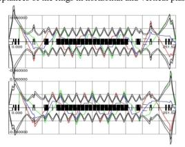
Figure 4: Scattered particles envelopes tracking. Beam envelopes (6 $\sigma$  and 7 $\sigma$ , black curves) are shown in horizontal (top) and vertical (bottom) planes.
