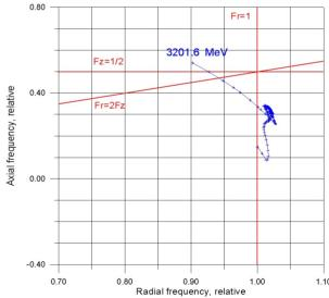
Figure 5: Phase diagram of Bi<sub>209</sub><sup>+43</sup> acceleration at the level of 700 kA turn.
