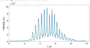
Figure 4: Bunch train structure inside VEPP-5 linac [8].
