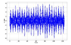
Figure 7: Vertical orbit distortions,  $\sigma_{x/y}$  is 50  $\mu m$
