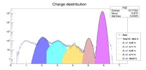
Figure 9: Carbon ion beam composition. 300 MeV/u.
