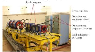
Figure 5: Electromagnetic scanning system.
