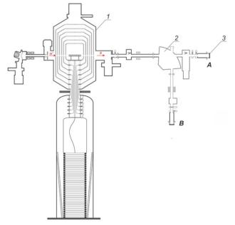
Figure 1: Tandem accelerator with vacuum insulation: 1 – accelerator, 2 – bending magnet, 3 – lithium neutron generating target. The lithium target is placed in the horizontal proton beam transport path (position A) or in the vertical (position B).
