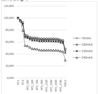
Figure 4: The efficiency of transmission of the <sup>48</sup>Ca<sup>10+</sup>.
