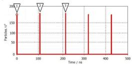
Figure 5: Distribution of beams at the cavity exit as a function of time, when the cavities are already filled.
