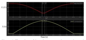
Figure 4: The values of the voltage across the capacitor and the current in the coil during the pulse.
