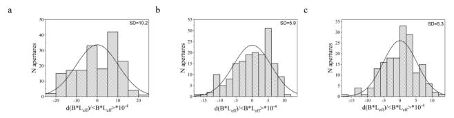
Figure 5: Distributions of relative deviation of the magnetic field integral for 2.3 kA (a), 6.89 kA (b) and 10.44 kA (c).
