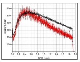
Figure 6:  $\langle RC(t)\rangle$  with the electron current off (black curve) and on (red curve). The electron energy is 1.78 keV, the electron beam current 150 mA. The latter is the optimum electron energy for electron cooling equal to  $(E_e)_{opt} = (m_e/m_{nucleon}) \times E_{ion}$ , where  $E_e$  is electron energy (not corrected to electron beam space charge potential!),  $E_{ion}$  is the ion energy per nucleon.
