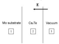
Figure 2: Photocathode model.
