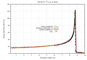
Figure 4: The total absorbed dose versus depth inside water phantom at 200 MeV/u of incident 12C beam  $(R_{csda}=8.575 \text{ g/cm}^2).$
