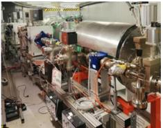
Figure 5: Transport channel HILAC-Booster.
