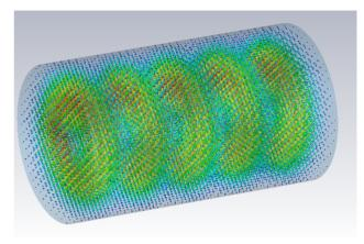
Figure 4: Cavity e- field distribution at selected size.
