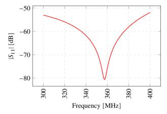
Figure 5: RF window reflection coefficient.
