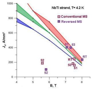
Figure 3: Current density  $J_e$  vs. magnetic field B in superconducting ECR magnets. S1, S2, S3 - solenoids, RT racetrack coil.
