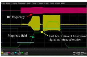
Figure 8: RF adiabatic voltage impact on the beam.
