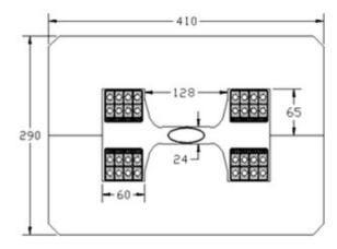
Figure 1: The dipole cross section.
