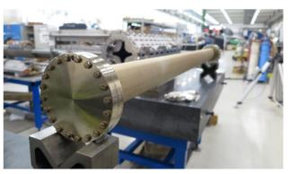
Figure 7: Checking the geometric parameters of the beam pipe and its further installation in a SC magnet.
