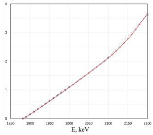
Figure 2: Dependence of the neutron yield Y on the proton energy E in the  $^7\text{Li}(p,n)^7\text{Be}$  reaction:  $\lozenge$  – from [3],  $\circ$  – calculated by the PINO program [4].
