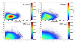
Figure 6: particle invariant distribution after 4-D painting injection.
