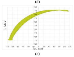
Figure 2: Calculated energy distributions in electron bunches after the first (a), second (b), third (c), fourth (d) and fifth (e) accelerating stage.
