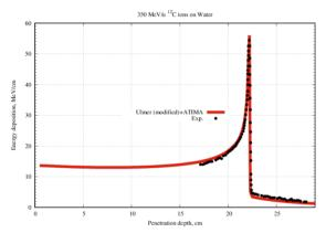
Figure 7: The total absorbed dose versus depth inside water phantom at 350 MeV/u of incident <sup>12</sup>C beam (R<sub>csda</sub>=21.872 g/cm<sup>2</sup>).
