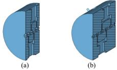
Figure 1: 3D models of the 80 MHz IH cavities.
