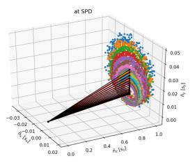
Figure 3: Mean spin-vector  $\langle s \rangle$  (or, what is the same, invariant spin axis  $\bar{n}$ ) orientations at the SPD-detector for particles with varying initial offsets from the closed orbit in the radial direction at injection. Colored dots indicate the ellipses the spin-vectors describe during precession.
