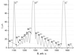
Figure 8: Bi ion spectrum. The operating mode is optimized to produce <sup>209</sup>Bi<sup>32+</sup>. Microwave power 221 W.
