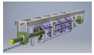
Figure 4: Serial magnetometer for FAIR quadrupole units.
