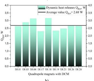
Figure 5: a) Experimental values of heat leak of quadrupole magnets of the Booster synchrotron with DCM; b) Experimental values of dynamic heat releases of quadrupole magnets of the Booster synchrotron with DCM.
