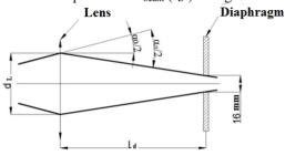
Figure 6:  $d_L$  is the diameter of the beam in the lens. D - measuring diaphragm with a hole diameter of 16 mm.  $D_{beam}$  is the beam diameter in the diaphragm,  $L_d$  is the distance from the lens to the diaphragm, which is 940 mm.
