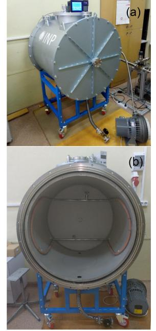
Figure 2: (a) Fabricated test cryostat, (b) the liquid nitrogen shield.
