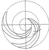
Figure 2: There is a difference between the sector length along the azimuth AB and the "effective" length A<sub>1</sub>B<sub>1</sub> at large spiraling angles. The effective width of the sector long the perpendicular to the sector centerline is equal  $A_1B_1 \approx AB \cdot \cos \gamma$ .
