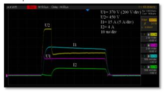
Figure 4: Oscillograms of voltage and current in auxiliary  $(U_2, I_2)$  and main discharges  $(U_1, I_1)$ .
