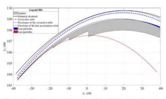
Figure 4: The estimated location of the ESD with a linearly decreasing electrostatic field for ion beam 209Bi38+.
