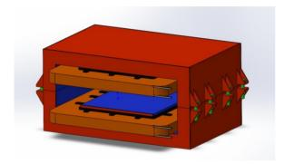
Figure 6: Dipole magnet 0.06 T.
