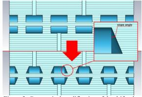
Figure 3: Geometrical modification of the drift tube.
