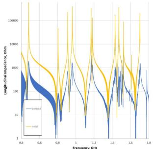
Figure 8: Comparison of the longitudinal shunt impedance for monopole HOMs for an initial accelerating cavity and with HOM waveguides.
