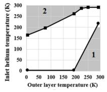
Figure 7: Admissible temperatures of the incoming helium flow Ti at cooling (•) and warming (•) of the quadrupole as a function of the temperature To of the outlet end of the outer layer. The outer shell is 1.4436 steel, the inner tube is 1.4571 steel. 1 - region of unacceptable temperatures of the input helium flow during cooling. 2 - region of unacceptable temperatures of the input helium flow during
