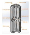
Figure 2: The Light Ion Linac SC cavity design.
