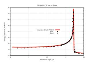
Figure 6: The total absorbed dose versus depth inside water phantom at 300 MeV/u of incident <sup>12</sup>C beam (R<sub>csda</sub>=16.983 g/cm<sup>2</sup>).
