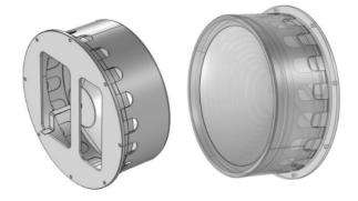
Figure 1: The cathode assembly.
