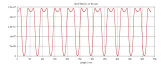
Figure 4: Electric field distribution of BAS structure consists of 10 sections.
