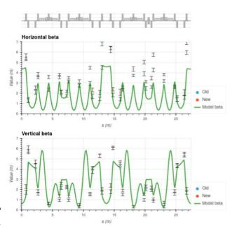
Figure 3: Measured (red points - after beam position correction, blue - before) and model beta-functions.
