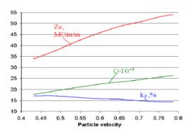
Figure 1: Comparison of the accelerating structures at 991MHz operating frequency.
