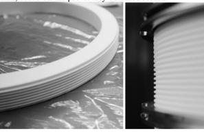
Figure 3: Ribbed ceramic surface 35 mm insulator (left) and 70 mm insulator (right) before training.
