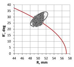
Figure 5: Radial position of 209Bi38+ beam at the entrance of puller (first acceleration gap).
