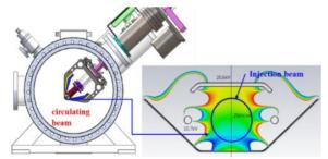
Figure 7: Corner septum cross section and its field map. A corner electrostatic septum is used to deflect the injection beam to the closed orbit, as shown in Fig. 7. The septum wire with the thickness of 0.1 mm is tilted by 40° to
