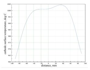
Figure 3: Cathode surface temperature distribution in horizontal section.
