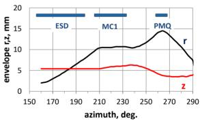
Figure 12: The radial and vertical envelopes of 209Bi38+ extracted beam.
