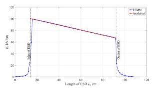
Figure 3: The amplitude value of the electric field strength along the central trajectory of the ESD.
