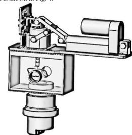
Figure 4: A prototype of low intensity beam control unit with removable film.
