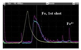
Figure 2: TOF spectrum of the ions at the output of the laser ion source, white vertical line is TOF marker for Fe<sup>16+</sup>, lilac - SEM detector signals, blue - collected signal at the SEM input, yellow - collected signal at the analyzer input.
