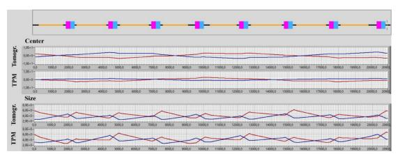
Figure 6: Scheme of the transport line around the matching cavity (on top) and beam position and size dynamics through the simulated transport line. On the scheme pink and blue rectangles are quadrupole lenses, orange lines are accelerating cavities, black lines are drift spaces. On the graphs blue lines are for the X-axis, red lines are for the Y-axis.
