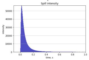
Figure 7: Spill structure for constant amplitude of RF-knockout.
