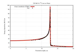
Figure 5: The total absorbed dose versus depth inside water phantom at 250 MeV/u of incident 12C beam  $(R_{csda}=12.527 \text{ g/cm}^2).$
