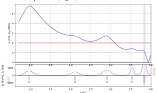
Figure 8: Resulting envelope and magnetic field longitudinal distribution.
