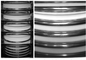
Figure 7: Ribbed ceramic surface (left, right) after training without breakdown traces.
