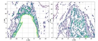
Figure 5: Dynamic aperture with errors.  $\sigma_{x/y}$  is 35  $\mu$ m on the left and 100  $\mu$ m on the right.
