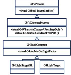
Figure 3: Inheritance diagram for GEANT4 classes describing ICS photon generation from the Light Target. The base class G4BackCompton inherits from G4VDiscrete-Process. G4LightTarget and G4LightTargetNL (not constructed yet) implement pure virtual function GetLightTarget for laser beam parameters transfer.
