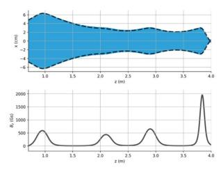
Figure 5: A comparison of simulations using the K-V envelope code (black dotted line) and REDPIC (blue filling). The bottom line shows the longitudinal distribution of magnetic field.
