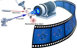
Figure 1: Scheme of operation of the TR-SFX method. Instead of an optical laser (Pump), there can be an X-ray pulse (the first pulse is Pump, and the second is Probe) [5].
