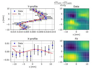
Figure 3: The result of the two-dimentional join fit to the left and right distributions of the scattered photons. The vertical (Y) projection shows Compton back scattering asymmetry due to vertical polarization of electron beam appearance
