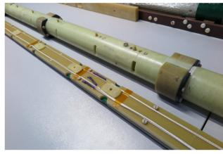
Figure 1: Magnetometer (lodgement and measuring shaft).
