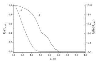
Figure 3: The calculated laser beam energy density distributions on the small mirror of the amplifier telescope. The spatial filter base detuning is +80 mm.
