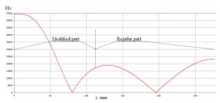
Figure 6: Dependence of tangential magnetic field component Hx along WG. Line x=0, y=0, see. Fig. 5.
