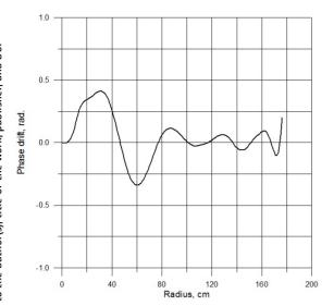
Figure 6: Calculated phase motion in the resultant magnetic field at the level of 700 kA turn.
