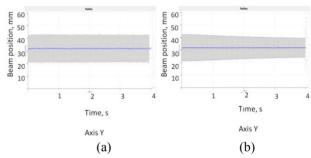
Figure 5: Y position of <sup>14+</sup>Fe beam as a function of time: (a) without electron cooling; (b) with electron cooling. The working electron cooling voltage is 1.83 keV.
