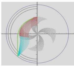
Figure 2: Trajectories of extracted beams.
