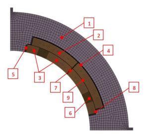
Figure 2: Finite element model in the first quadrant of the coil block. 1- collar, 2- outer coil layer, 3-inner coil layer, 4- protective metal gasket, 5- end metal gasket, 6- separator, 7- body insulation, 8- inner spacer, 9- interlayer gasket.
