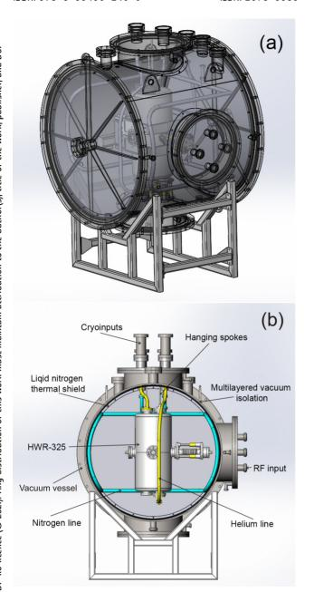
Figure 1: (a) The sketch of test cryostat model with a cavity inside, (b) the main parts and subsystems of the cryostat.
