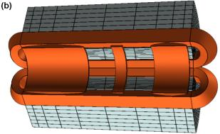
Figure 2: Reversed (solenoid-in-sextupole) magnetic system. Model without (a) and with (b) iron.
