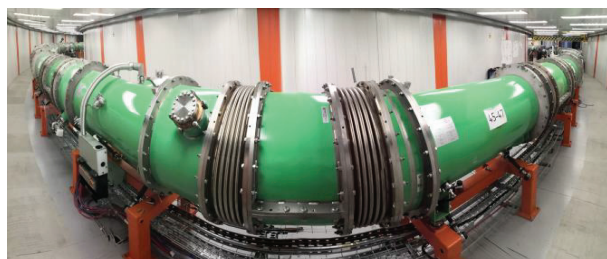
Figure 2: Booster ring in the tunnel inside the Synchrotron iron yoke.
