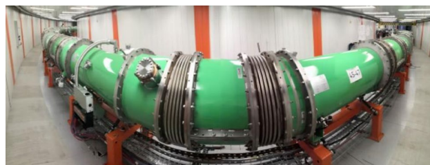
Figure 7: Booster ring inside Synchrohasatron yoke.
