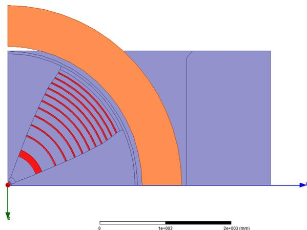
Figure 1: 3D calculation model of 1/8 part of the magnet.
