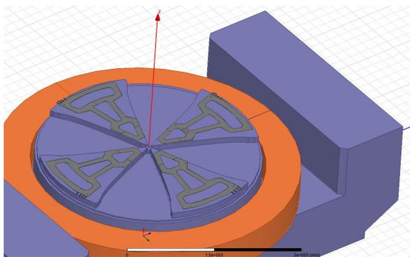
Figure 3: 3D calculation model of 1/2 electromagnet with azimuthal coil housings.
