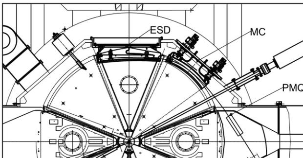
Figure 1: Layout of the elements of extraction system.
