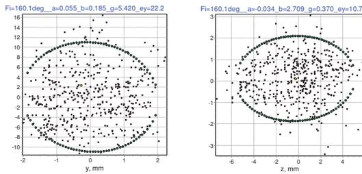
Figure 3: The horizontal and vertical beam emittances at the deflector entrance (A/Z=5.5, B<sub>0</sub>=1.55 T).
