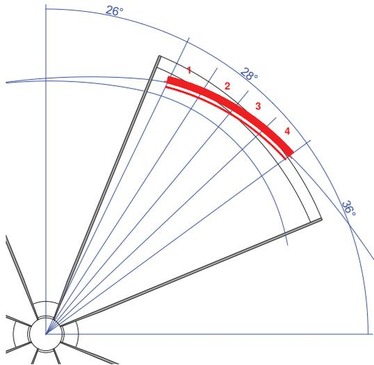
Figure 7: Layout of the magnetic channel in the cyclotron extraction system.
