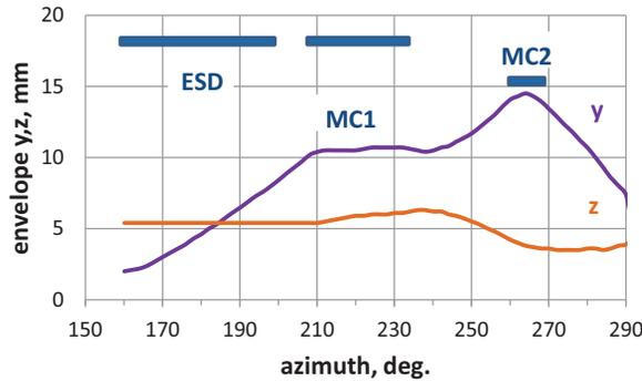
Figure 4: The horizontal and vertical beam envelopes.
