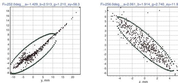
Figure 5: The horizontal and vertical beam emittances at the PMQ entrance (A/Z=5.5, B<sub>0</sub>=1.55 T).
