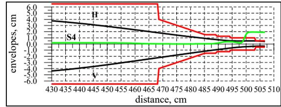
Figure 9: Envelopes of  $\text{Au}^{26+}$  ion beam near inflector.
