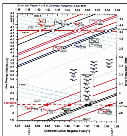
Figure 1: Working diagram of DC140 cyclotron.
