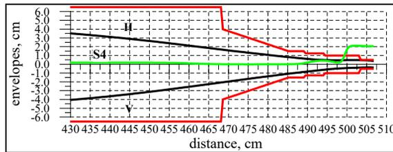
Figure 7: Envelopes of  $\text{Bi}^{38+}$  ion beam near inflector.
