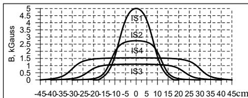
Figure 3: On-axis magnetic field of solenoids.
