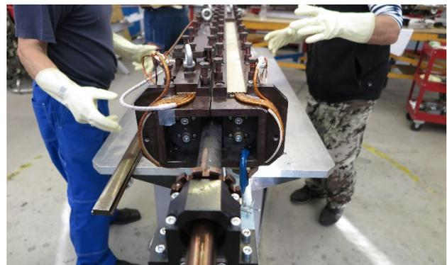
Figure 3: Equipment for baking the SC winding for the NICA collider dipole magnet.
