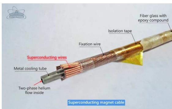
Figure 1: View of the hollow SC cable.
