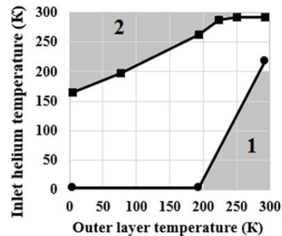
Figure 7: Admissible temperatures of the incoming helium flow  $T_i$  at cooling (●) and warming (■) of the quadrupole as a function of the temperature  $T_o$  of the outlet end of the outer layer. The outer shell is 1.4436 steel, the inner tube is 1.4571 steel. 1 - region of unacceptable temperatures of the input helium flow during cooling. 2 - region of unacceptable temperatures of the input helium flow during warming.
