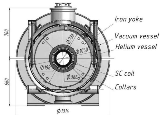
Figure 1: Cross section of the quadrupole FFS.
