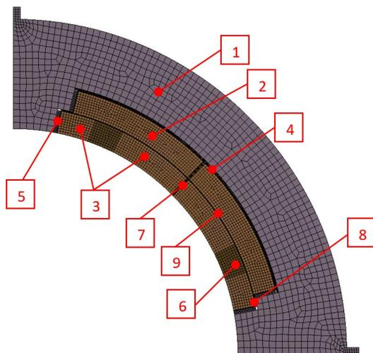
Figure 2: Finite element model in the first quadrant of the coil block. 1- collar, 2- outer coil layer, 3-inner coil layer, 4- protective metal gasket, 5- end metal gasket, 6- separator, 7- body insulation, 8- inner spacer, 9- interlayer gasket.
