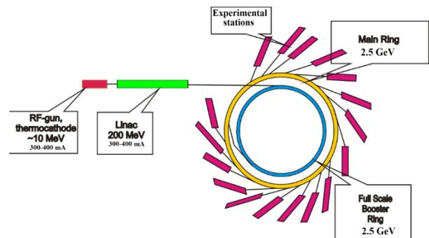
Figure 1: Planned scheme of the accelerator complex.
