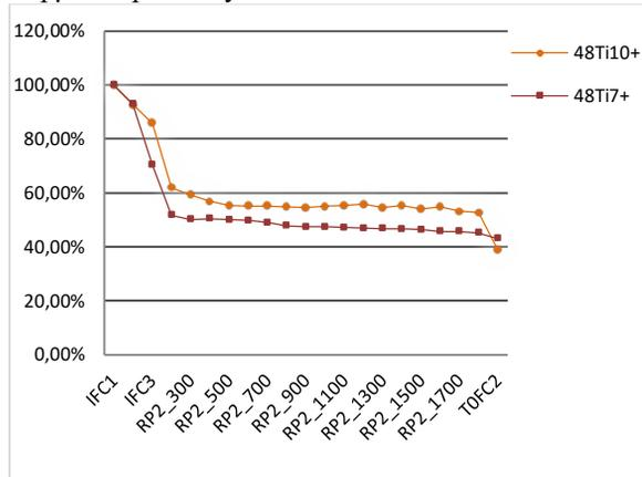
Figure 5: The efficiency of transmission of the  $^{48}\text{Ti}^{10+,7+}$ .
