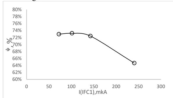
Figure 3: The efficiency of capture into acceleration.
