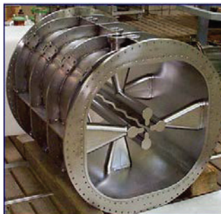
PIAVE SRFQ – first (and alone) superconducting RFQ, LNL INFN
