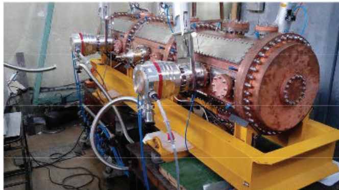
RFQ linac with RF and vacuum components installed on resonator in tuning area (ITEP)
