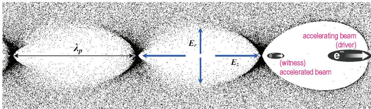
Proton drivers: 20 kJ (SPS), >150kJ (LHC) drivers have enough energy in a single bunch to accelerate electrons to TeVs in a single plasma stage
