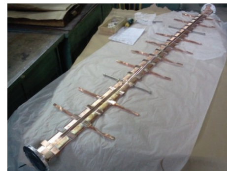
Magnetic system of 72-pole indirect cooling 3Tesla wiggler for CLIC dumping ring.
