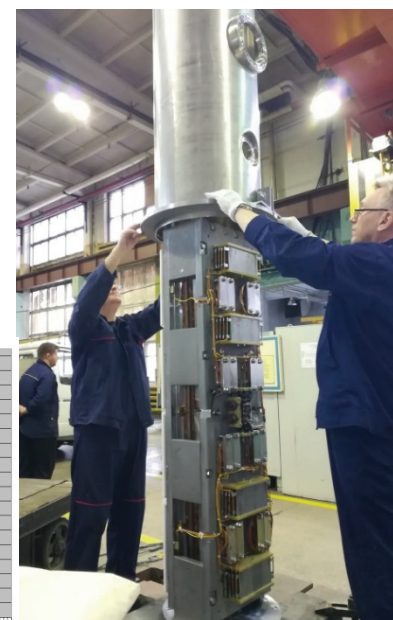
Inserting SC magnet to Lhe vessel
