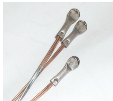
Cold welded connection with resistance of 10^{-13} Ohm
