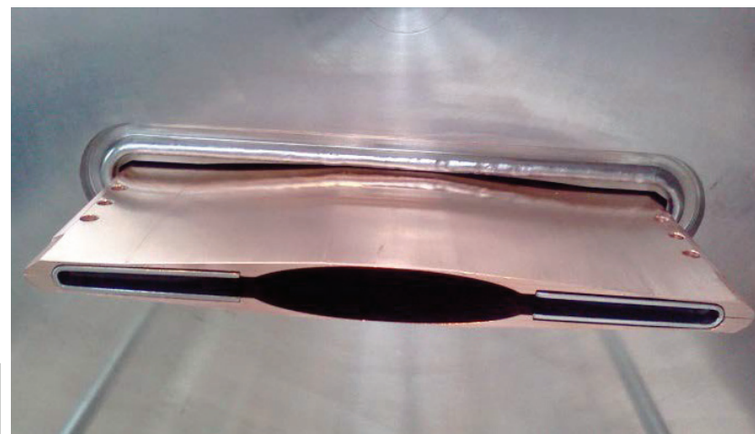
Design of magnetic gap of LSU-CAMD 7T 15-pole SCW. (Horizontal aperture 200 mm, vertical gaps between chambers \sim 0.5 mm along of \sim 2 m) (2015)
