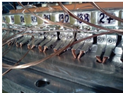
Magnetic system of 72-pole indirect cooling 3Tesla wiggler for CLIC dumping ring.
