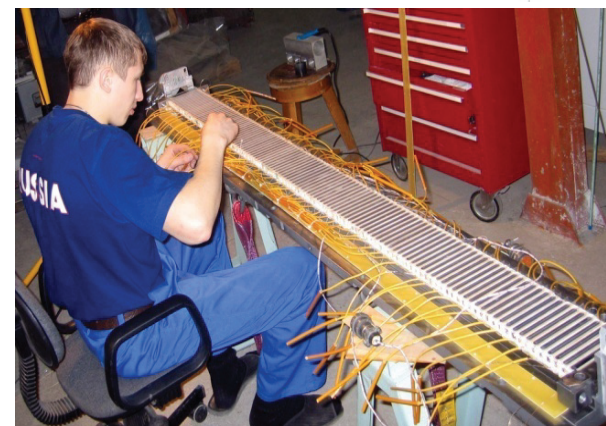
Short period magnet array of horizontal racetrack type poles (for ALBA 2.1 T SCW with 30 mm period)
