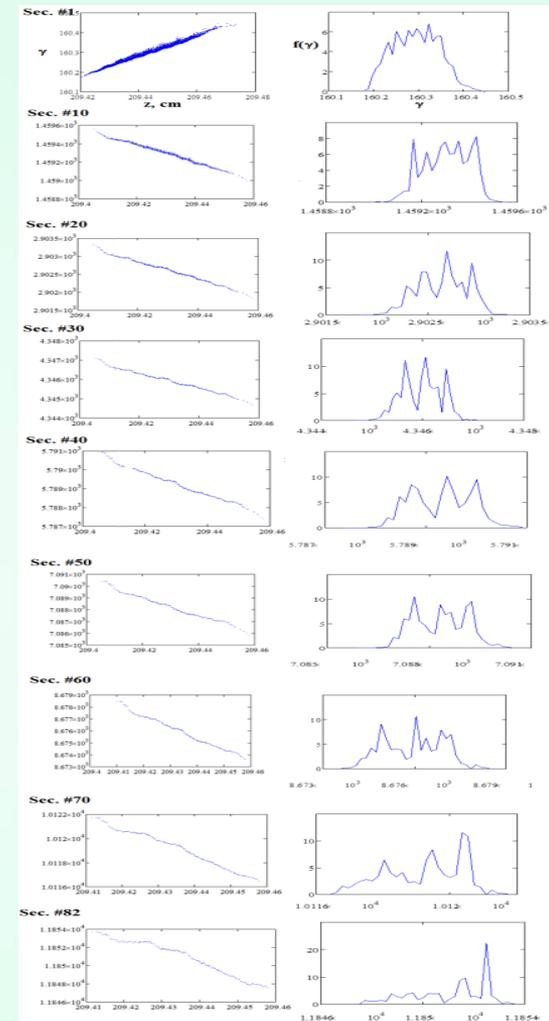
Beam dynamics simulation results for 40-cell BAS and 250 pC bunches: longitudinal phase spaces on the  $(\gamma, z)$  phase plane and energy spectrums.
