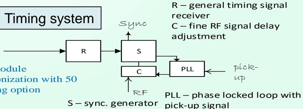
*BPM module synchronization with 50 ps timing option*
