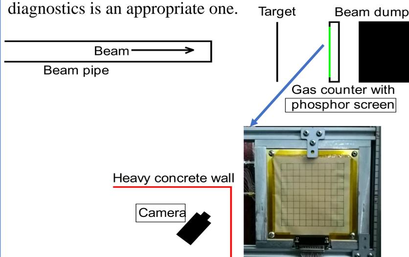
Fig. 1. Layout of luminescent diagnostics components and phosphor screen at INR PIF.
