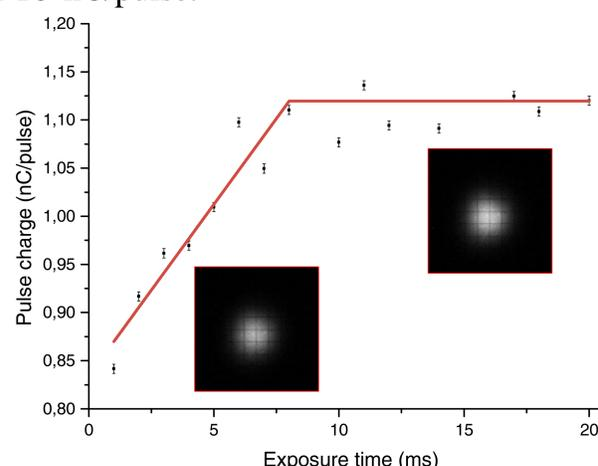
Fig. 6. Dependence of measured pulse charge on camera exposure.
