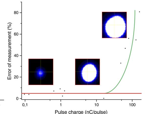
Fig. 7. Dependence of measurement error on pulse charge.
