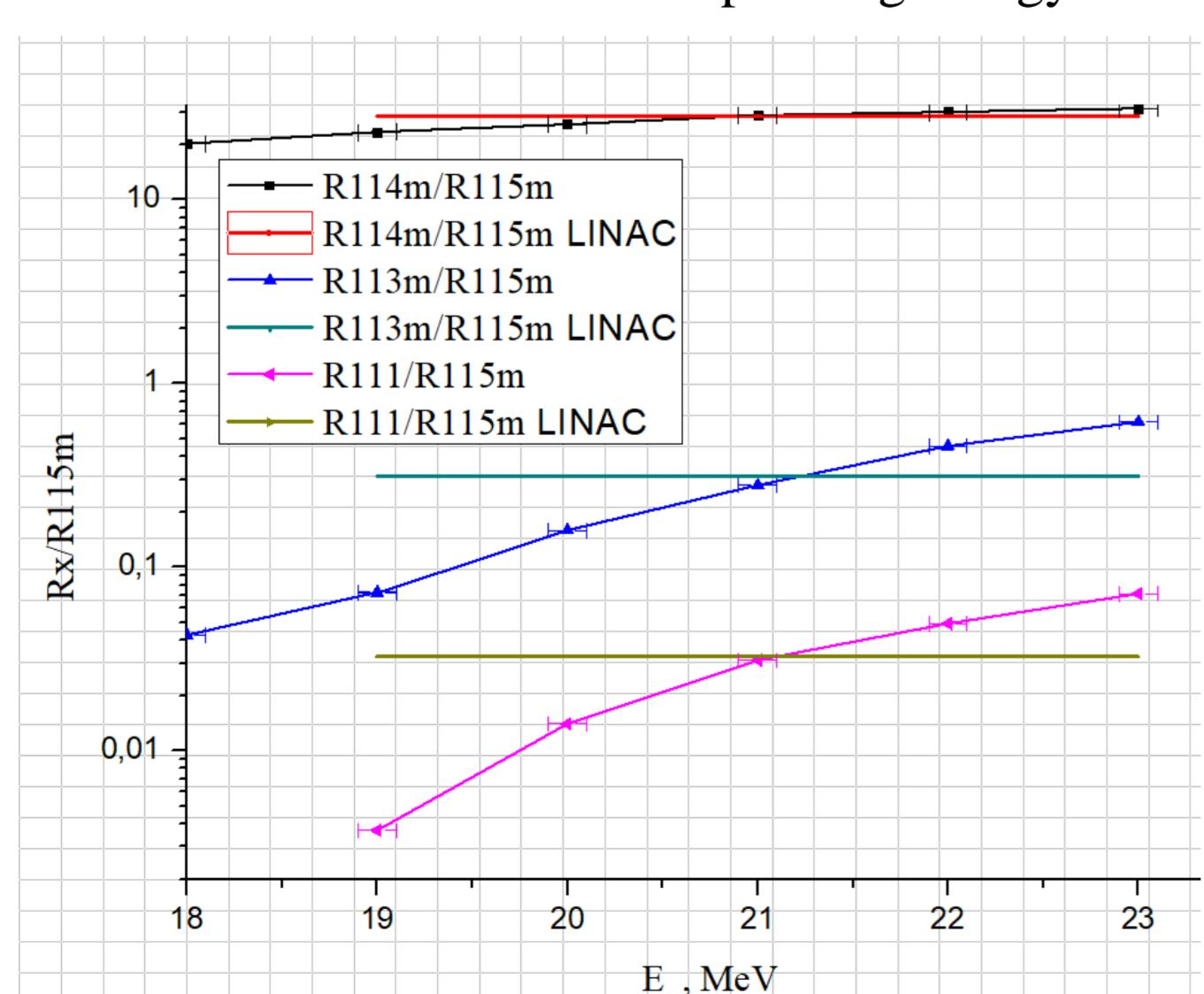
Energy of  $21\pm0.1$  MeV measured on LINAC by the ratio of different isotopes of indium.
