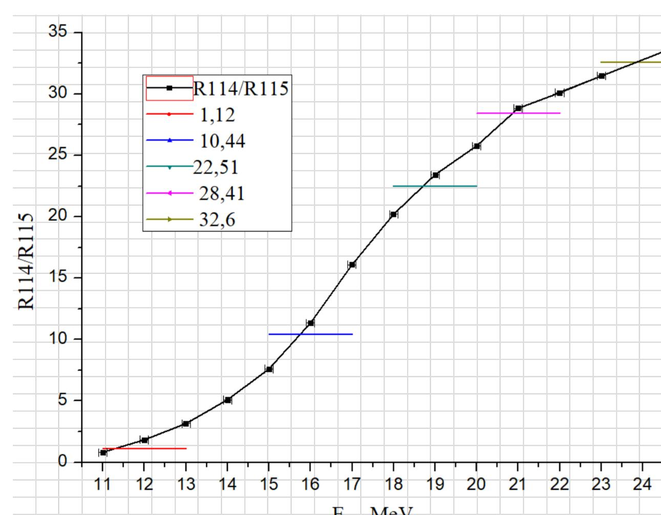
Dependence of the ratio of the activity of indium isotopes  $^{114}\text{In}/^{115}\text{In}$  on the energy of electrons accelerated on a microtron. (the lines show the ratio of the activity of indium isotopes measured on LINAC and the corresponding energy value)
