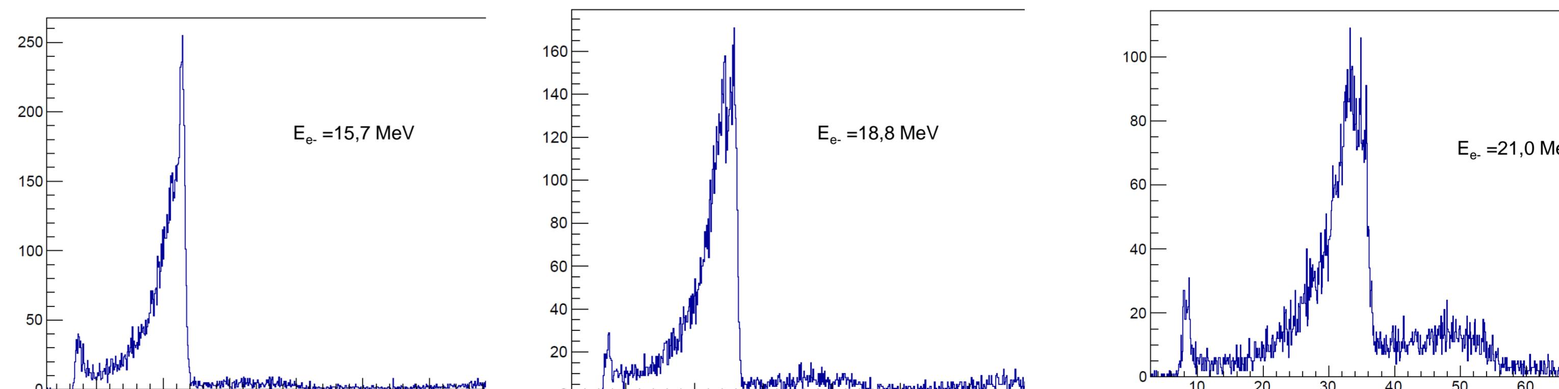
Single-electron spectra measured by scintillation detector BGO on LINAC
