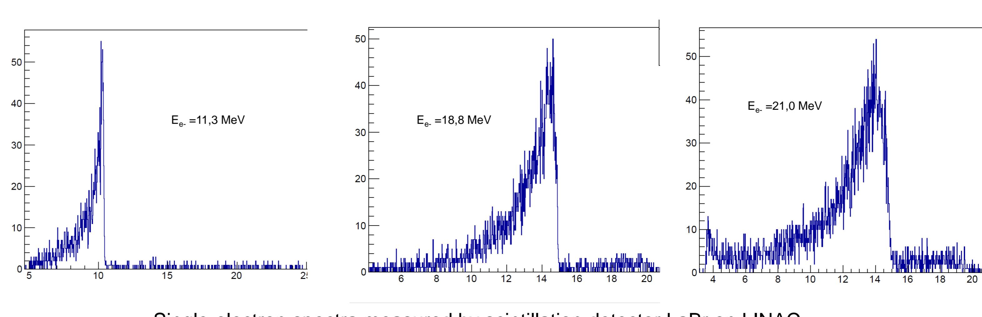
Single-electron spectra measured by scintillation detector LaBr on LINAC
