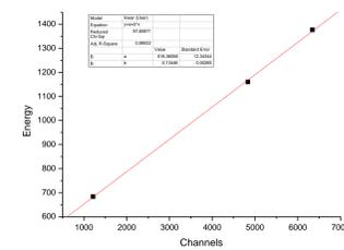
The energy of Xe ion beams as a function of the channel number
