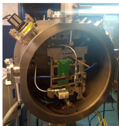
Detectors in the test chamber
