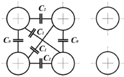
Figure 2. Capacitances of accelerating channel
