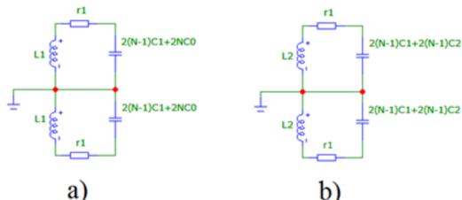
Figure 3. Equivalent circuits of the accelerating structure in synchronous and in non-synchronous modes
