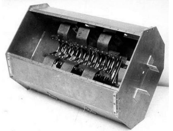
Figure 7. The mock-up of the accelerating structure with the electrostatic undulator
