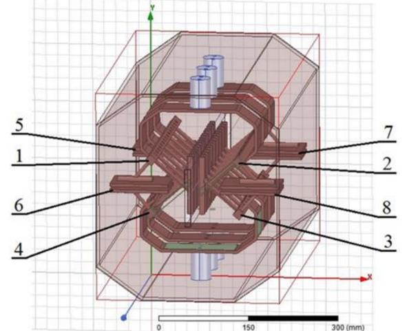
Figure 8. The HFSS model of the accelerating structure with the corrective capacitors
