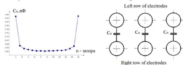
Figure 4. Capacitance distribution in the accelerating channel
