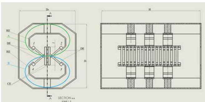
Figure 1. The design of the accelerating structure
