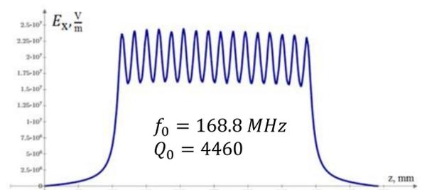
Figure 9. The distribution of electrical component of RF field after installation of corrective capacitors
