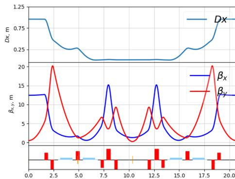
Figure 3: Lattice functions in 67 nm-rad operation mode.
