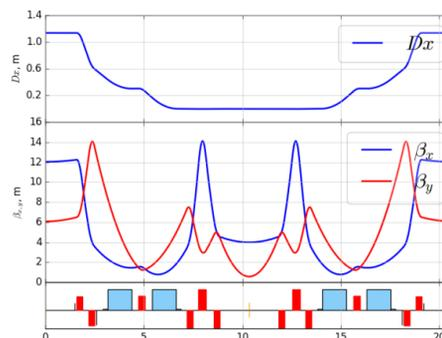
Figure 1: Lattice functions in user operation mode.
