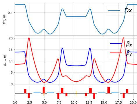
Figure 5: Lattice functions in 17 nm-rad operation mode.
