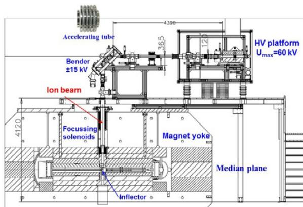
Figure 6: Scheme of the DC280 axial injection.
