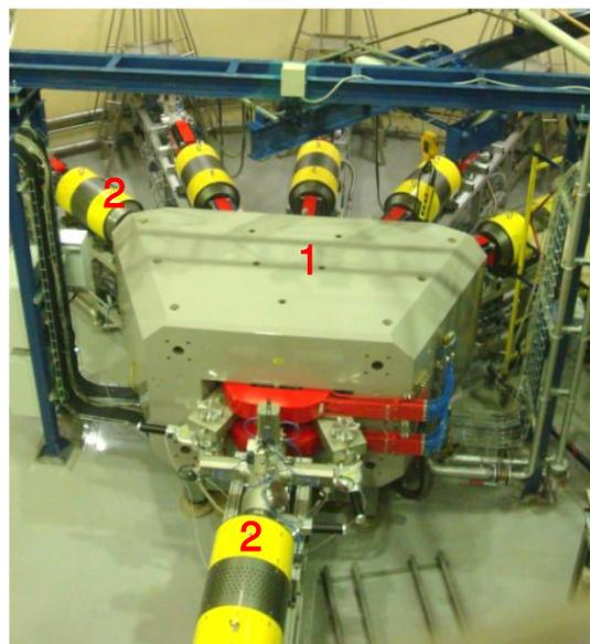
Figure 14: Beam transport channels, where: 1-  $\pm 50^\circ$  bending magnet, 2- quadrupole lenses.
