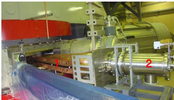
Figure 11: Flat-top resonator, where: 1 - dee with plating, 2- resonator.
