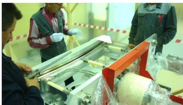
Figure 12: Electrostatic deflector.
