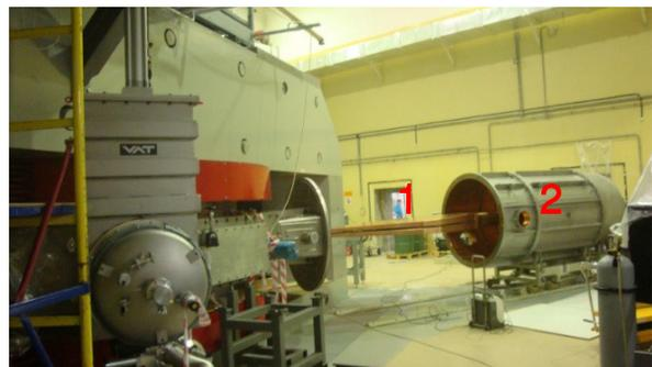
Figure 10: Main resonator with dee, where: 1 - dee, 2- resonator.
