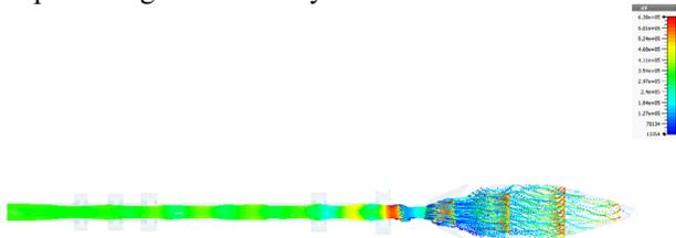
Figure 1: Dynamics of a beam in a klystron.
