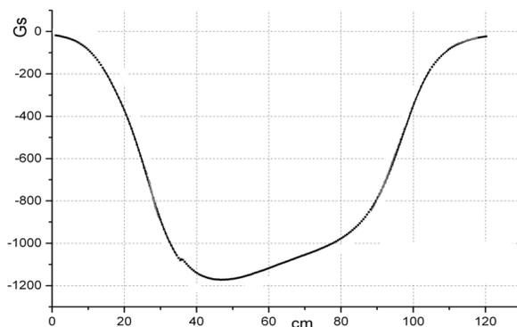
Figure 4: Magnetic field on the axis of the solenoid.
