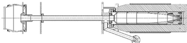
Figure 3: Model for testing the cathode node and collector.
