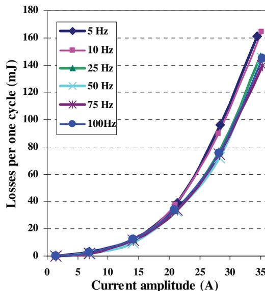
Figure 2: Dependence of AC losses on current in AMSC coil without the iron core.
