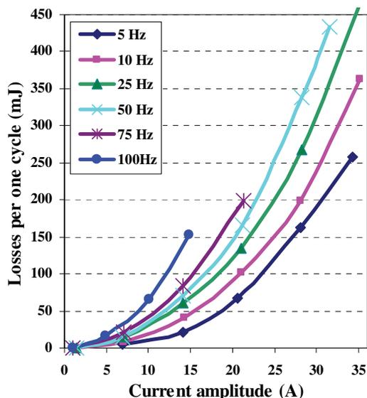
Figure 4: Dependence of AC losses on current in AMSC coil with the iron core.
