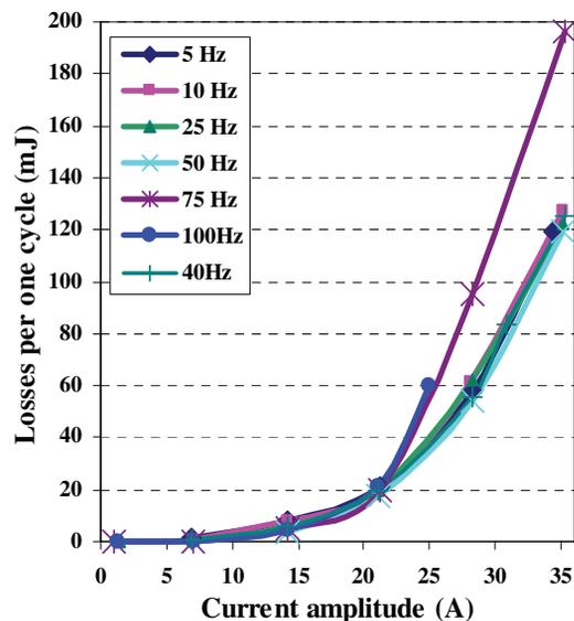
Figure 3: Dependence of AC losses on current in SuperOx coil without the iron core.
