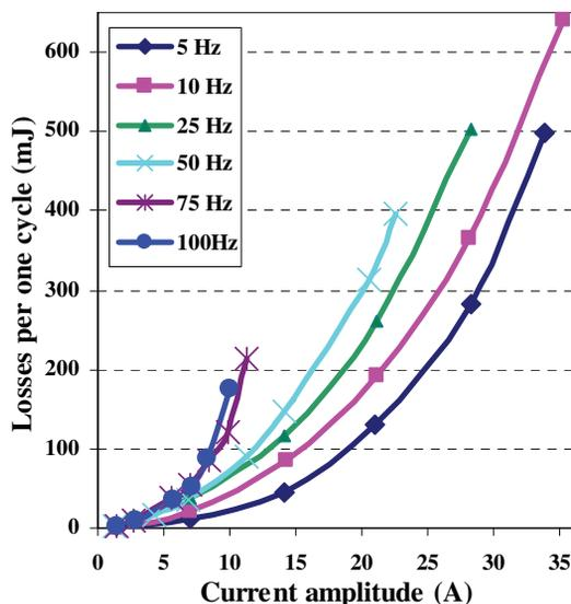
Figure 5: Dependence of AC losses on current in SuperOx coil with the iron core.
