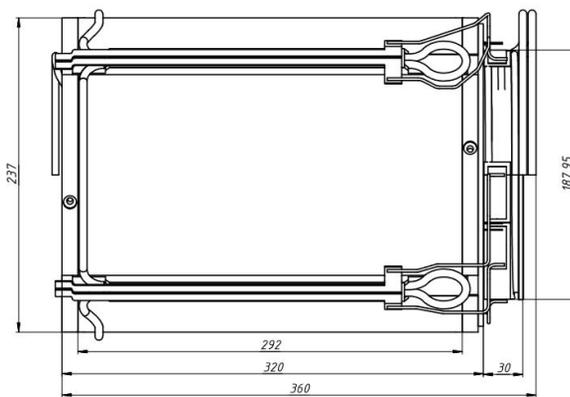
Figure 2: Main view of the multipole magnet.
