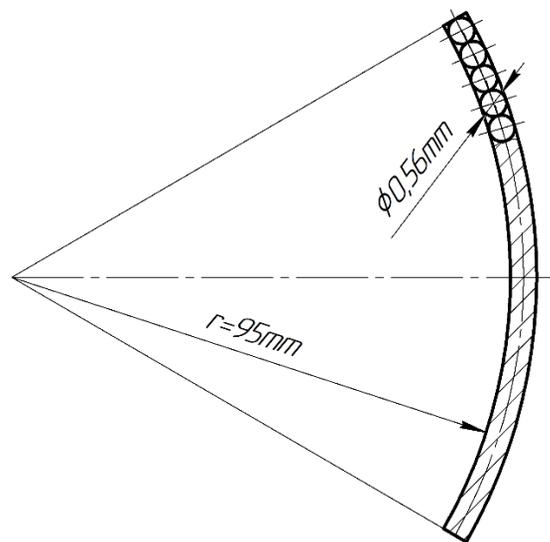
Figure 3: Coil cross-section.
