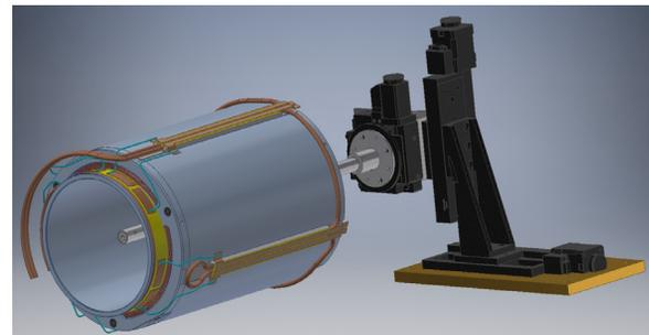
Figure 6: Layout of the magnetic measurement system.
