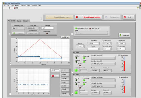
Figure 6: The program for automation of dynamic heat releases measurement: 1 - Controlling buttons, 2 - Measurement status bar, 3 - Status of energy evacuation switch, 4 - Data graph, 5 - Cycle parameters, 6 - Heat releases power graph, 7 - Status of first power supply, 8 - Status of second power supply.
