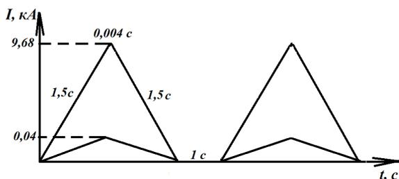
Figure 7: Quadrupole magnet's current cycle.
