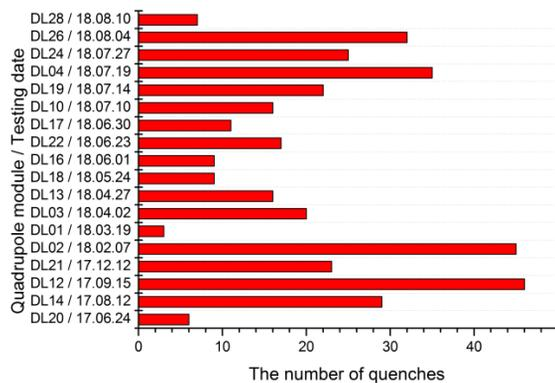
Figure 2: Quenches quantity of the quadrupole doublets.
