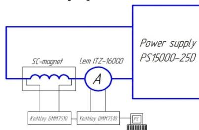
Figure 5: The scheme of dynamic heat releases measurement.
