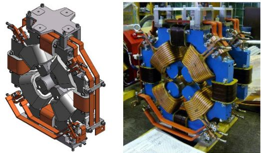
Figure 8: Quads 3D-model (left) and the result (right).
