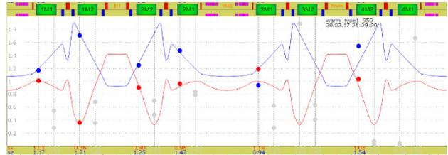
Figure 14: Model (solid lines) and measured (dots) horizontal (red) and vertical (blue) beam sizes at 940 MeV in "new warm" regime.
