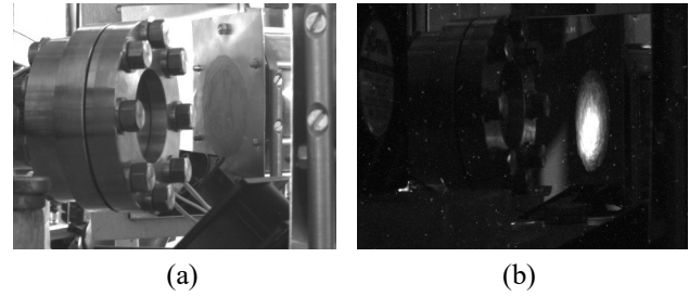
Figure 5: Image of the plate with luminophor: with no beam (a), with a beam (b).
