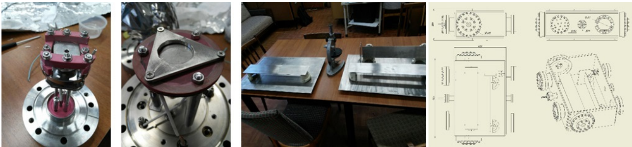
Figure 2: The gun, holder of the sample, the setup under assembling, scheme of the setup.
