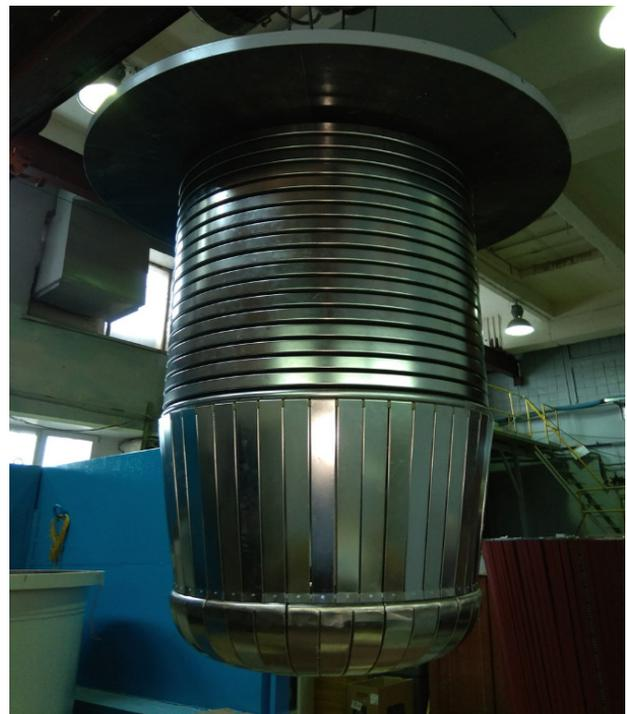
Figure 5: Photo of the rectifier column.
