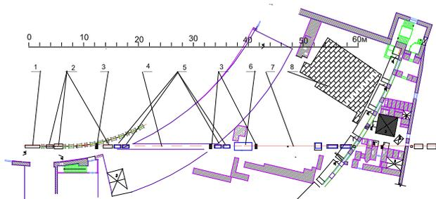
Figure 1: The place for new channels location . 1 – septum magnet, 2 – magnets for bend extracted ion beam in vertical plane to the top, 3 – devices of JNIR PIK for measurement shape of the beam, 4 – beamline with angle 0.105 to the top, 5 – existing quadrupoles, 6 – magnet SP12, 7 – beamlines in horizontal direction, 8 – concrete walls.
