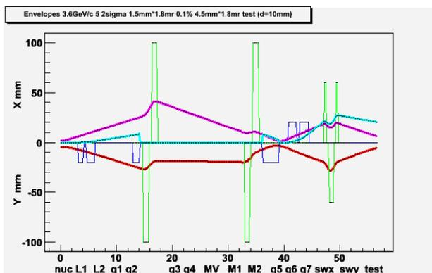
Figure 6: Beam envelopes scheme for bend at 24 degree at beam diameter like 10mm.
