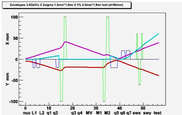
Figure 5: Beam envelopes scheme for bend at 24 degree. X – horizontal plane, Y vertical plane, blue – positions of magnets, green – positions and apertures of quadrupoles.
