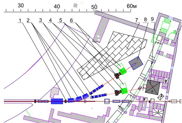
Figure 4: Layout of channels at three bends on 12 degrees. 1 – PIC4, 2 – magnets, 3 – triplets and scanning magnets on common supports, 4 – devices and collimations, 5 – stands, 6 – entrance for montages, 7 – entrance for rooms, 8 – beam stop 2, 9 – old beam stop.
