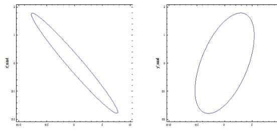
Figure 2: Phase volumes of extracted beams at level  $2 * \sigma$ .
