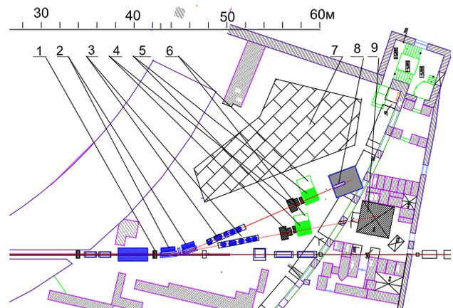
Figure 3: Layout of channels at two bends on 12 degrees. 1 – PIK4, 2 – magnets, 3 – triplets and scanning magnets on common supports, 4 – devices and collimations, 5 – stands, 6 – entrance for montages, 7 – entrance for rooms, 8 – beam stop 2, 9 – old beam stop.
