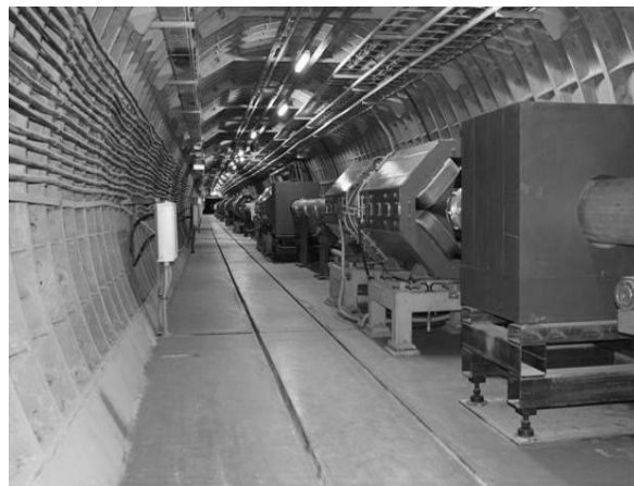
Figure 1: Section of PRGC-100 with quadrupole lenses and radiation protection blocks.
