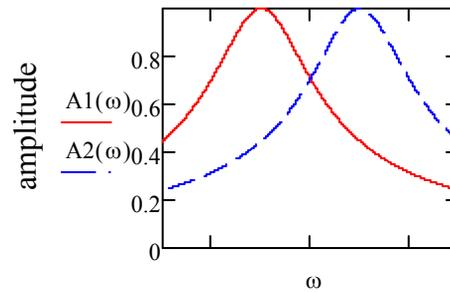
Figure 1: Zero and  $\pi$  modes two coupled cavities.
