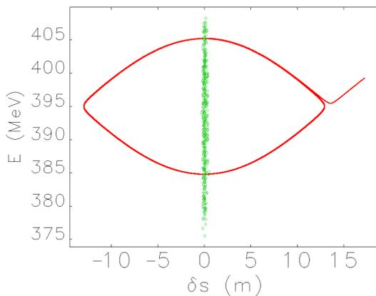
Figure 6: Damping Ring separatrix with injected beam.
