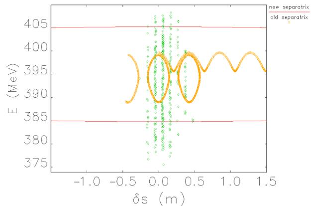
Figure 7: Injected beam in energy separatrix before and after RF-system upgrade.
