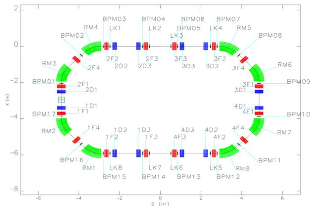
Figure 2: Damping Ring layout.
