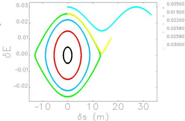
Figure 4: Phase trajectories for synchrotron oscillations.
