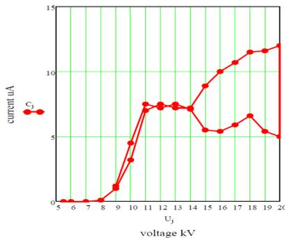
Figure 3: The corona current versus voltage.
