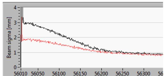
Figure 1: The proton beam cooling at COSY (Juelich). The cooling time is about 100 s.
