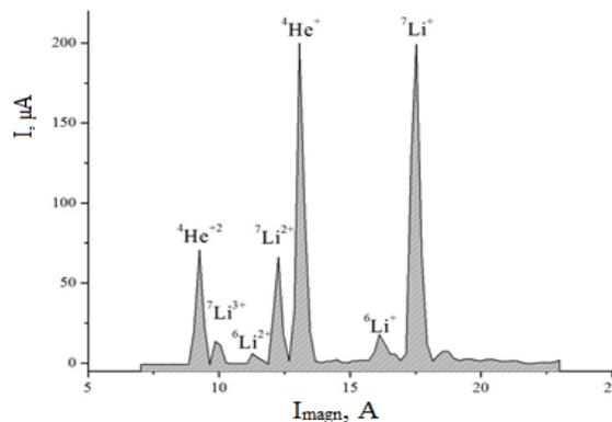
Figure 5: Charge state distribution of the extracted Li ions with the enlarged crucible (EC).
