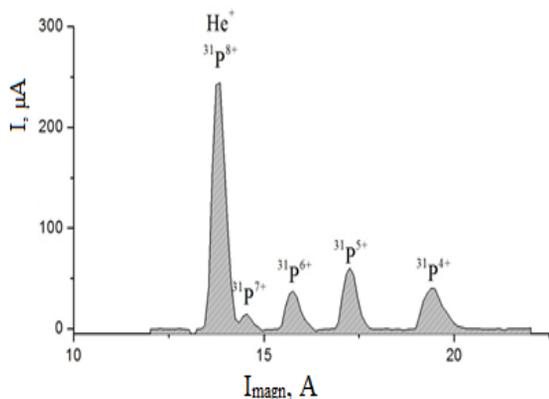
Figure 9: Charge state distribution of the extracted P ions (SC).
