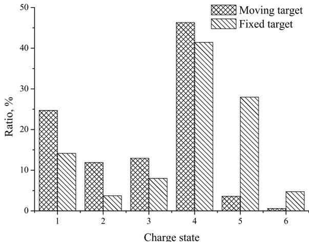
Figure 7: Charge state distributions measured with fixed and moving target.
