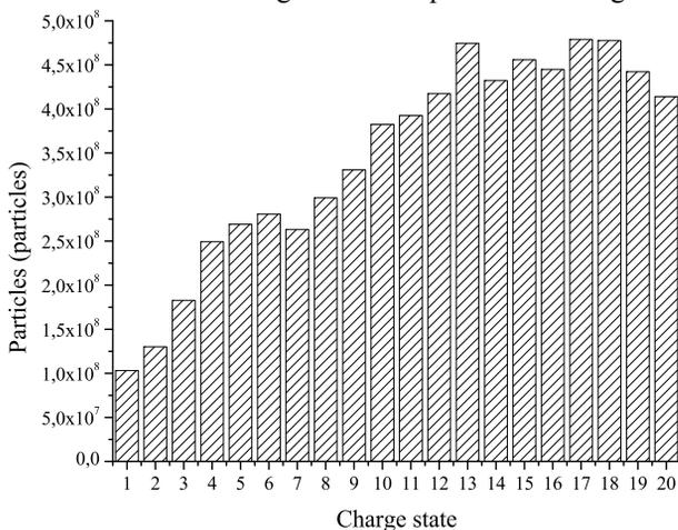
Figure 8: Charge state distribution in tungsten ion plasma.
