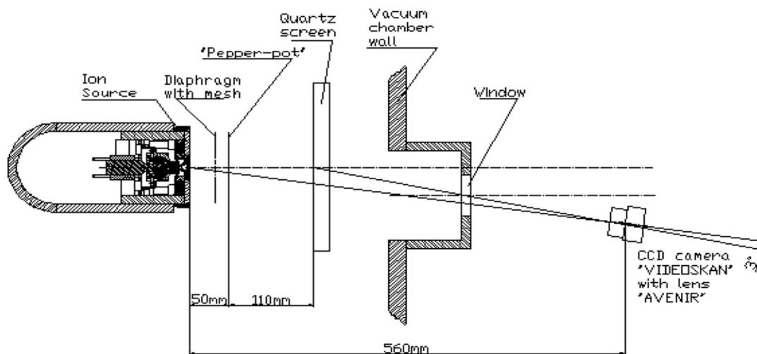
Figure 1: Scheme of the emittance measuring device.
