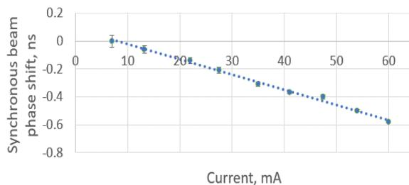
Figure 10. Synchronous beam phase shift vs. current.
