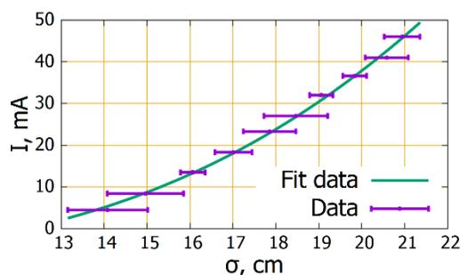
Figure 5: Longitudinal beam size vs. beam current (streak-camera).
