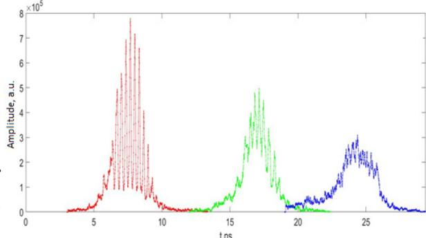
Figure 3: Specific beam grouping stages (red – 5<sup>th</sup> turn, green – 25<sup>th</sup>, blue – 115<sup>th</sup>).
