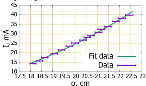
Figure 6: Longitudinal beam size vs. beam current (dissector).
