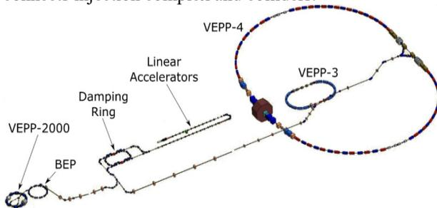
Figure 1: BINP's accelerator facilities layout.
