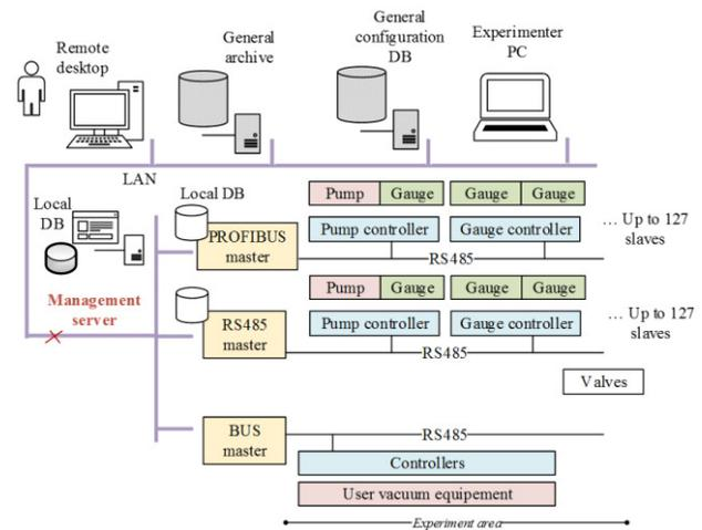
Figure 2: SSRS-4 Control System architecture.
