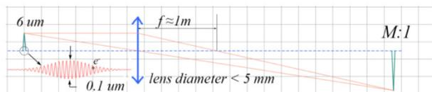
Figure 3: The X-ray optical system layout for the beam profile measurements.
